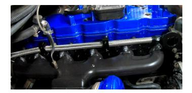
STEP 14: Ensure that the coolant drain plug has been reinstalled in the radiator and proceed to re-fill the cooling system. Re-use or replace coolant as necessary to properly fill the system with clean fluid.
