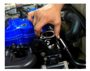
STEP 5: Place the stock thermostat housing over the thermostat riser block. Using the supplied M6 flange head bolts (item 6), tighten the bolts to 89 in-lbs.
