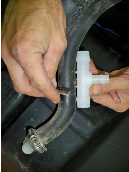
(Fig. 6) Cut 3/4" vent line hose approximately 4 1/2 inches from elbow end of hose.
