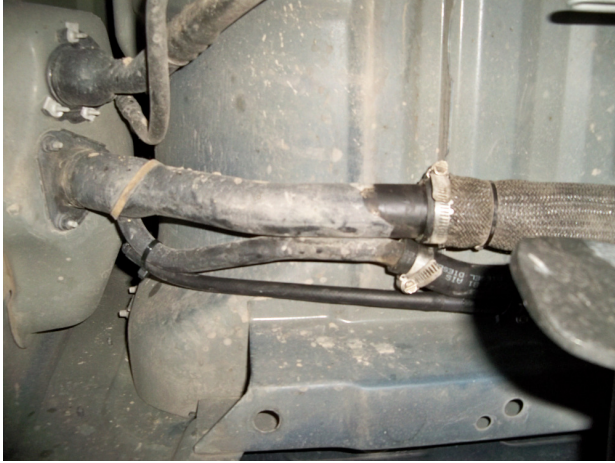
(Fig. 16) Attach fill and vent hoses, and attach hose from the Vacuum Vent Assembly as high as possible on vent tube with cable ties.
