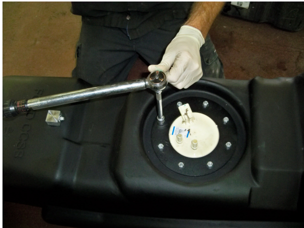
(Fig. 5) Using a torque wrench, tighten the top flange nuts to 20 ft. lbs. using a “star” pattern.
