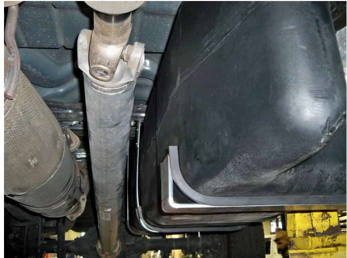
(Fig. 15) Installation of front support on tank without TITAN Shield. Note the rubber bushings on the support and the straps.
