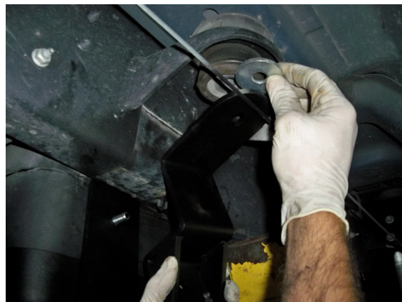
(Fig. 11) Place the supplied fender washer into the center of the rubber cab mount above the upper piece of the assembly.
