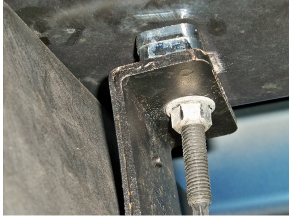
(Fig. 9) Tighten the bolt and bracket against the shims. If the strap does not hold the tank tightly enough, remove one shim at a time until it is tight.
