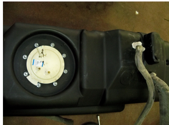
(Fig. 4) Be sure the sending unit is “clocked” the same as in the original equipment tank.
