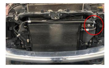
STEP 11: With the cooler lines routed and retained, tighten each of the four cooler line fittings to 270-350 in-lbs. Use a backup wrench on the fitting installed in the housings of the transmission cooler and transmission to prevent over torqueing.
