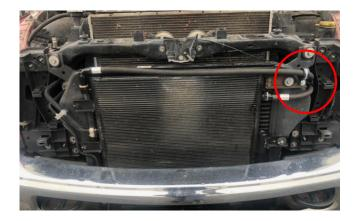
STEP 11: With the cooler lines routed and retained, tighten each of the four cooler line fittings to 270-350 in-lbs. Use a backup wrench on the fitting installed in the housings of the transmission cooler and transmission to prevent over torqueing.
