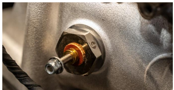
Figure 38: New heater with included M5 nut, used to retainer new heater harness.
