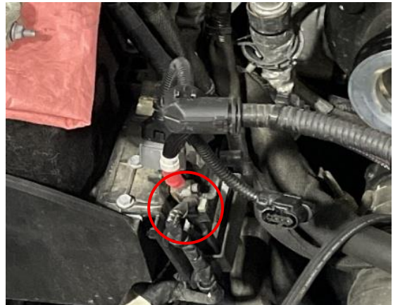
Figure 37: New heater harness installed on grid heater relay. 13mm nut reinstalled to retain new harness.
