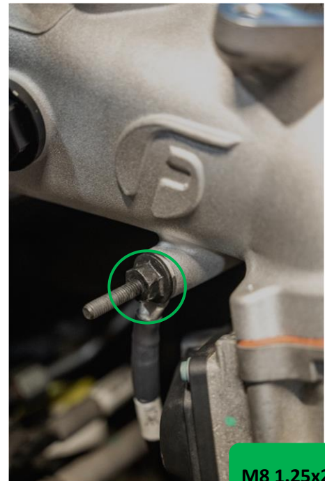
Figure 41: Heater ground cable installed at intake horn.
