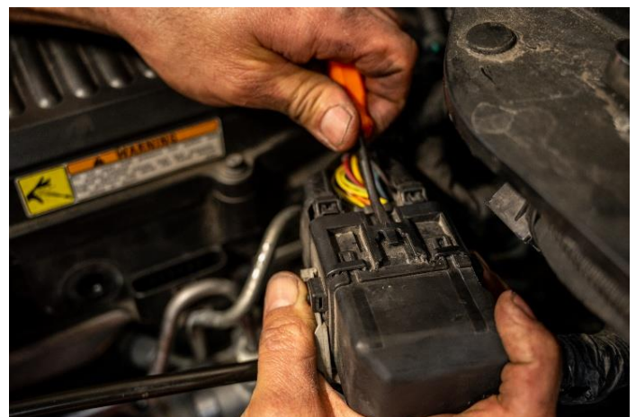
Figure 15: Removal of bulkhead at fire wall.
