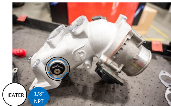
Figure 32: Heater plug and 1/8" NPT installed.
