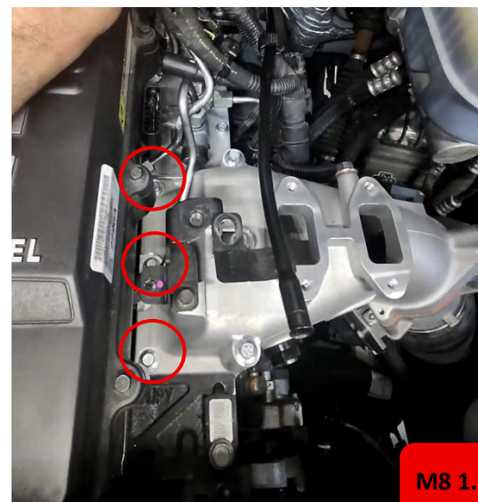
Figure 34: Three M8 1.25x35 bolts installed.
