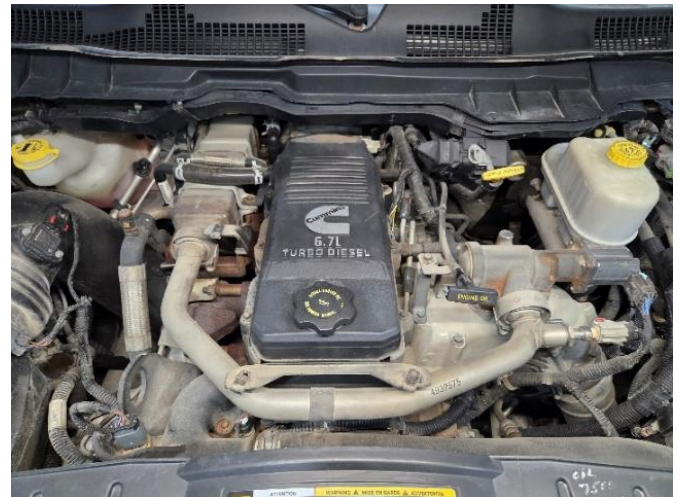
Figure 43: EGR Crossover tube reinstalled Model Years 2013-2018.
