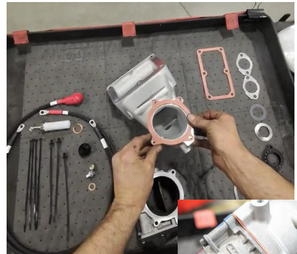
Figure 30: Installation of new throttle valve gasket. New intake horn and throttle valve assembled.
