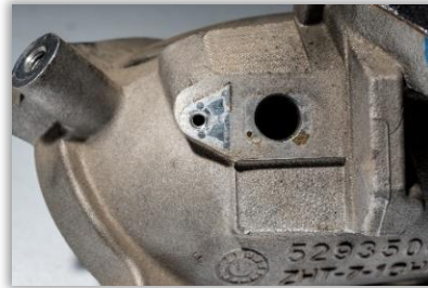
Figure 8A: MAP sensor location on intake horn.
