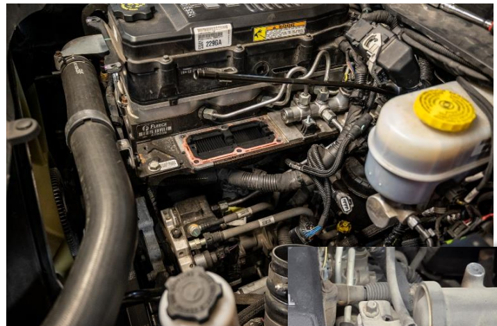
Figure 9: Stock intake horn and throttle valve removed.
