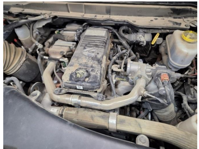
Figure 44: EGR Crossover tube reinstalled Model Years 2019-2024
