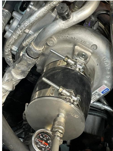
Figure 40: Boost leak tester installed.
