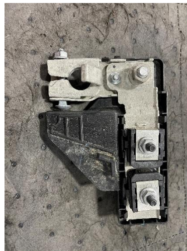
Figure 10: Positive terminal cluster removed.
