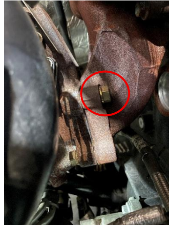
Figure 28: Turbocharger mounting location, mounting nut circled.
