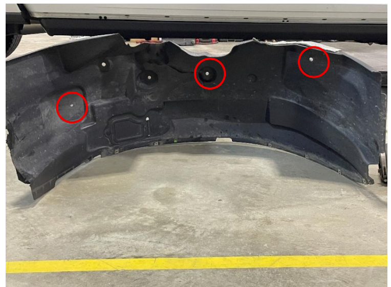
Figure 7B: Push Pin locations circled.
