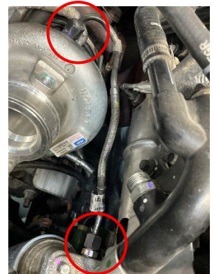
Figure 22: Oil feed line ends circled.
