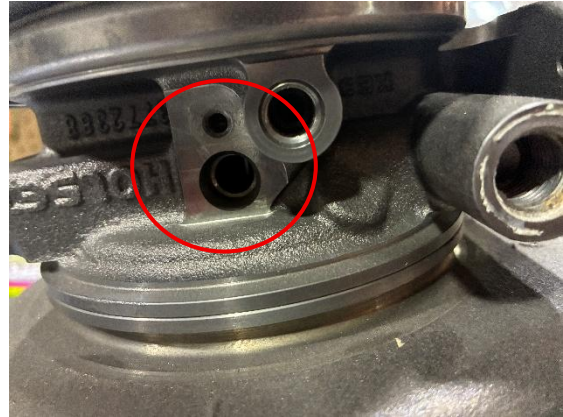
Figure 31: Mounting bore for speed sensor circled.
