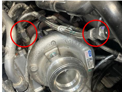
Figure 21: Coolant feed line ends circled.
