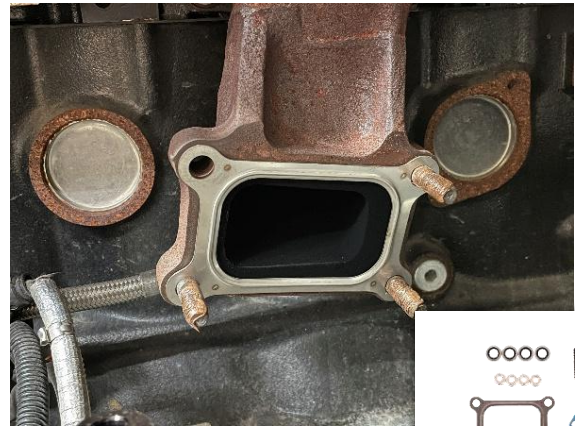
Figure 34: Flange gasket installed onto the exhaust manifold. Installation kit at right.
