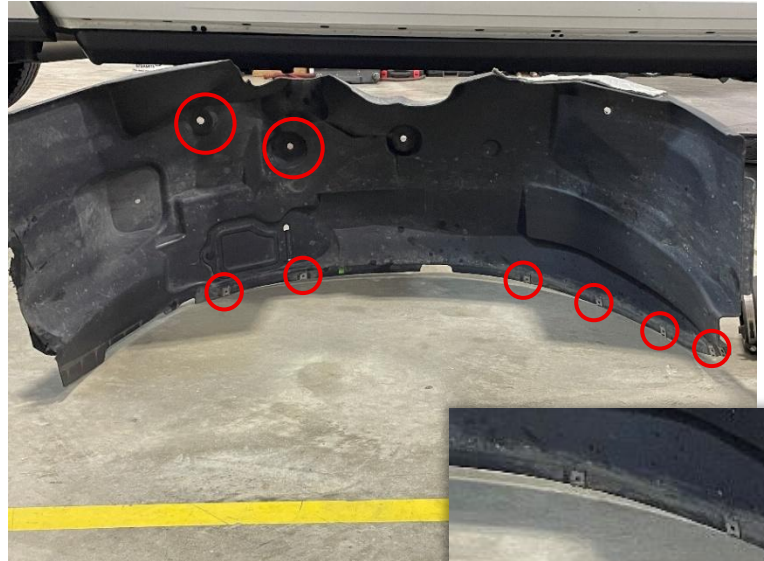
Figure 7A: Bolt locations on fender liner.
