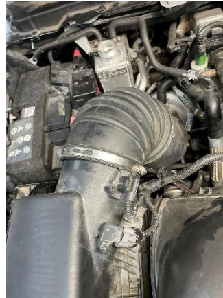
Figure 4A: Air intake tube before removal.
