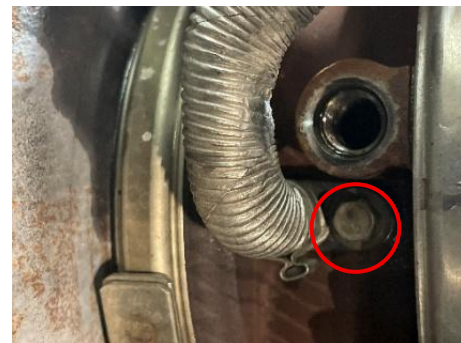
Figure 23: Turbine shaft speed sensor installed in turbocharger. 8MM bolt retaining the sensor circled.
