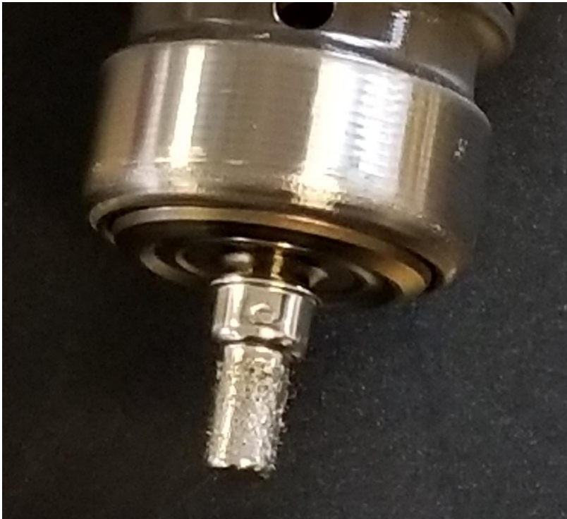
Figure 6: This is why we recommend replacement. This came out of a running truck with a CP4. Notice all the fine metal fragments imbedded in the filter.
