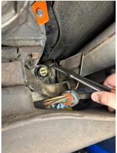
**STEP 5:** Remove the transmission pan using a 13mm socket.
