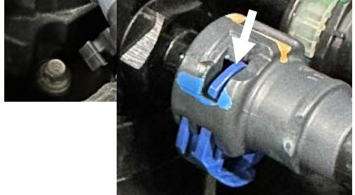
**STEP 2.1:** Remove the fuel output line first. This will be the left side quick disconnect with a blue locking tab. To release the blue locking tab, press both sides of the locking tab in the opposite direction of the filter housing and then into the fitting to release the tab.
