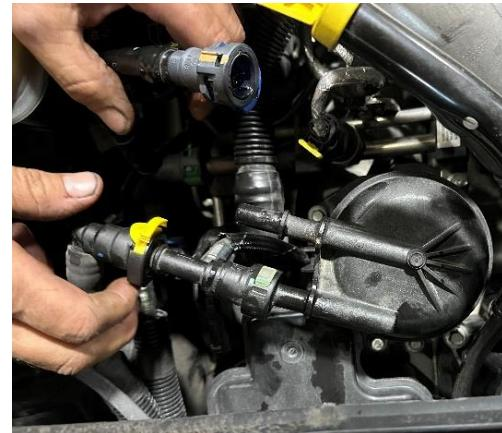
**STEP 4:** Install the new Fleece Performance filter bypass assembly into the filter mounting canister on the engine. Make note of the alignment dowel on the new filter bypass assembly and the locking tab position in the mounting canister. Align the locking tab and rotate the assembly clockwise into the housing.
