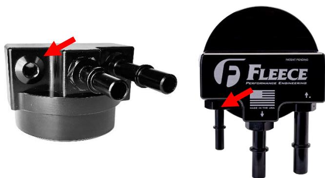
**STEP 5:** Install the new Fleece Performance filter bypass assembly into the filter mounting canister. Make note of the alignment dowel on the new filter bypass assembly and the position in the mounting canister. Align the locking tab and rotate the assembly clockwise into the housing.
