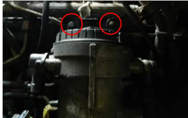
STEP 8: Remove the fuel filter assembly
