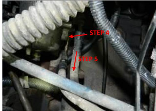
STEP 4: Disconnect the fuel feed line from the back of the fuel filter.
