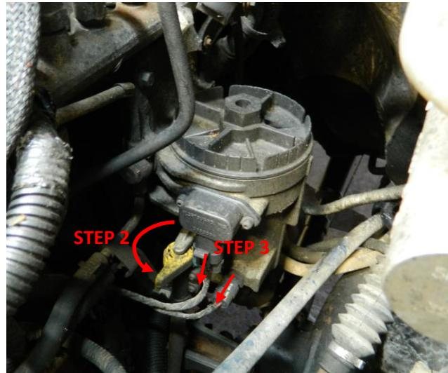
STEP 3: Unplug the fuel heater and WIF (water in fuel) sensor from the front of the fuel filter assembly.
