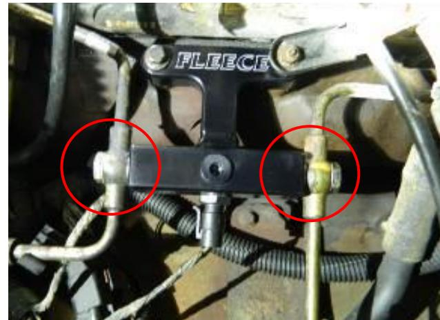
STEP 13: Tighten the fuel filter delete fasteners and torque the banjo bolts to factory spec's.
