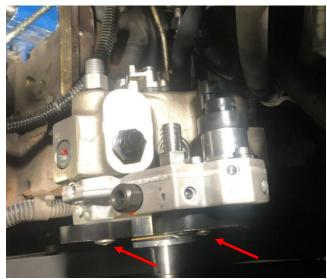
STEP 16: Locate the ½" pushlock hose you installed to the distribution block in STEP 12 and route it neatly alongside the engine and up to the 2<sup>nd</sup> pump. Cut it to length and install it onto your FPE high flow feed fitting. Using the -6AN 120 degree fitting thread it onto the return side of your 2<sup>nd</sup> pump and neatly route the %" pushlock hose you installed to the AUX port of the distribution block, cut it to fit and install the remaining -6AN 90 degree fitting.
