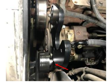
STEP 13: With the bracket securely mounted, install the idler pulley (item 3), aluminum spacer (item 4) and M10 x 40mm bolt (item 8) into the threaded hole in the pump bracket and tighten with a 15mm socket.
