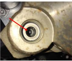
STEP 6.3: Remove spring from the plug and re-install onto the high pressure CP3 fitting.
