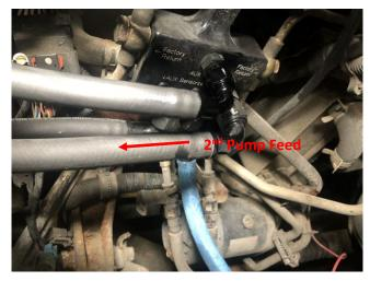
STEP 17: Install your high pressure CP3 to CP3 hard line (item 6), use a 19mm wrench to tighten to 17 ftlbs.
