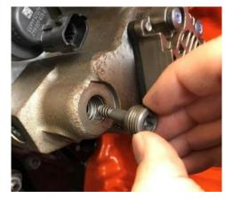
STEP 6.2: Ensure the check ball remains seated in place and does not fall out.
