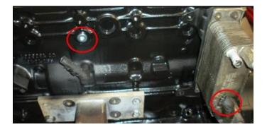
FPE-2018-03 October, 2018 Page 2 of 7 STEP 6: Using an 8mm Socket, remove the three bolts anchoring the stock thermostat housing. It is not necessary to remove or disconnect the thermostat housing from the upper radiator hose. Move it to the side, out of the way of the exposed thermostat, to allow for access.
