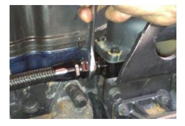
STEP 16: Utilizing the coolant bypass line riser brackets (item 11) and M8 socket head cap screws (item 5) in your kit; position the clamps over the bypass coolant line and fasten them to the cylinder head in the available tapped holes between cylinder numbers 2 & 3 as well as between cylinder numbers 4 & 5.
