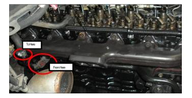
STEP 4: Install the provided heater tube and heater hose along with hose clamps (items 9, 12, and13) from the passenger side heater tube outlet to the factory 90° heater hose on the firewall. Use the supplied vinyl coated P-clamp (item 14) to secure the line.
