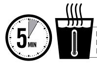
FOR PROPER INSTALLATION, SOAK AIR LINE TUBE ENDS IN HOT WATER BEFORE INSTALLING ONTO BARBED FITTINGS.
