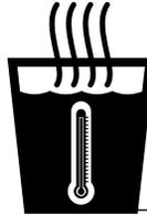
FOR PROPER INSTALLATION, SOAK AIR LINE TUBE ENDS IN HOT WATER BEFORE INSTALLING ONTO BARBED FITTINGS.
