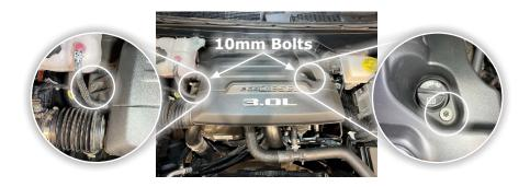
**STEP 3** - Remove the Intake Tube by loosening both hose clamps at both ends with an 8mm socket/wrench. Then, use a 10mm socket to remove the bolt holding down the Intake Tube.
