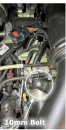
**STEP 4** - Use a clip removal tool to disconnect the Coolant Overflow Hose from the Intake Tube.
