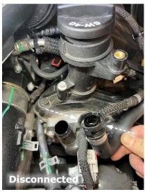
**STEP 7** - Remove the Intake Tube from the Airbox and Intake Inlet and set it aside.
