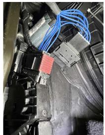
NOTE - If needed, use a flat head screwdriver or pick tool to gently pry the locking tab out.
