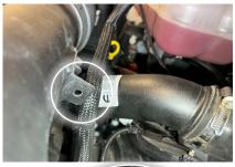
STEP 5 - Lift up on the Intake Tube to separate it from the Charge Pipe below it, the ball socket joint should come apart.
