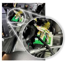
**STEP 18** - Plug the Pulsar XT module into the Pulsar XT connector until it clicks. Then, tuck the module behind the driver's side kick panel so that it is snugly held in place.
