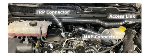
**STEP 10** - Disconnect both the MAP (Mass Air Pressure) Sensor and FRP (Fuel Rail Pressure) Sensor by first pushing back on the red locking tab and then pushing in on the release tab. Connect both sensors into the Pulsar XT harness.
