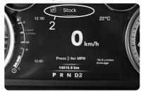
**STEP 1** - To change the power levels, use the RES+ and SET- buttons while cruise control is off. The level will briefly appear then disappear in the radio station slot.
