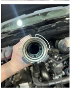
NOTE - To remove the Spring Clip, push the charge tube in towards the cab. Then, pull on both sides until they click into their respective latches. The Spring Clip should then unlock, freeing the Charge Pipe.
