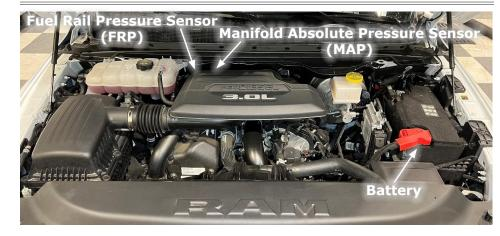
**STEP 1** - Disconnect the negative terminal on the battery using a 10mm socket/ wrench.
