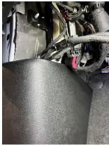
**STEP 19** - Use provided zip ties to secure excess cables away from the brake and accelerator pedals, hot surfaces, and any moving components in the cab and in the engine bay.
