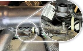
**STEP 6** - Disconnect the electrical connector on the PCV (indentified below), and then remove the PCV Hose from the Intake Tube by first locating the side connected to the engine and then squeezing in the sides of the lock ring and lifting up until the PCV Hose is disconnected.
