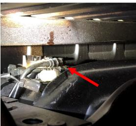
STEP 3: Remove the cross-member located at the front of the fuel tank. There will be 4, 15mm bolts to remove.
