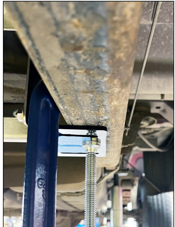
INSIDE / BRACKET EXTENDED AWAY FROM FRAME
