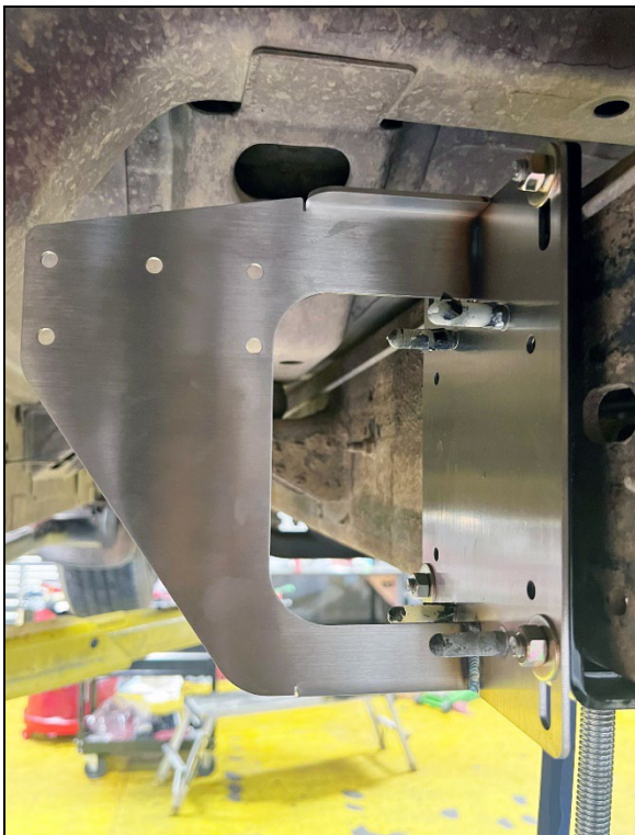
OUTSIDE / TIGHT TO FRAME / LOW POSITION
