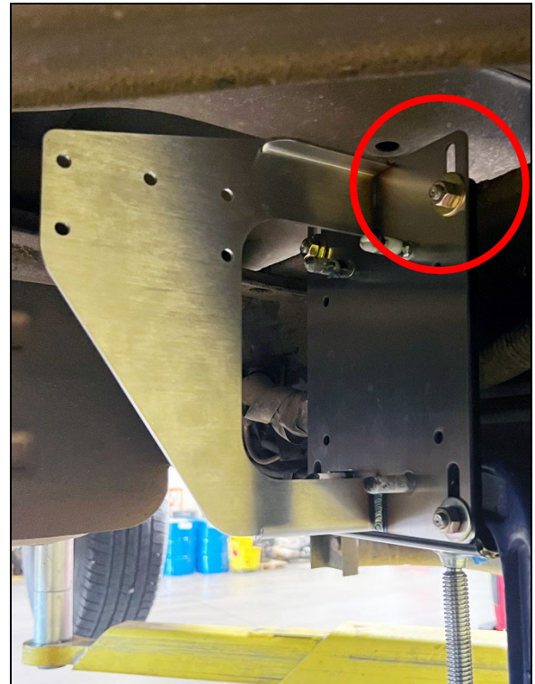
INSIDE / TIGHT TO FRAME / HIGH POSITION
