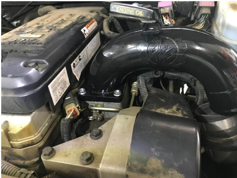
7. With the factory bolt fasten the dip stick bracket.
