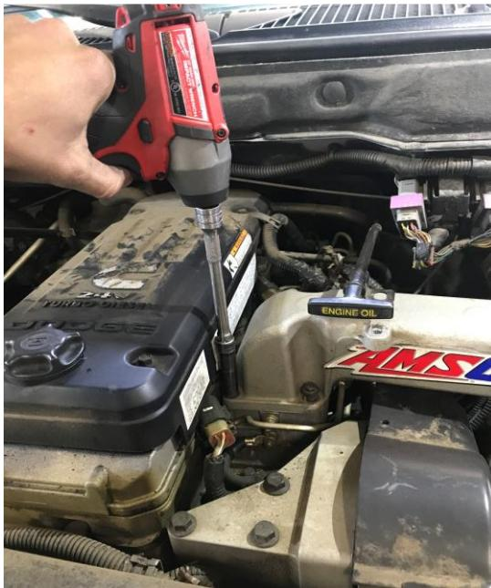
4. Now remove the intake elbow.
