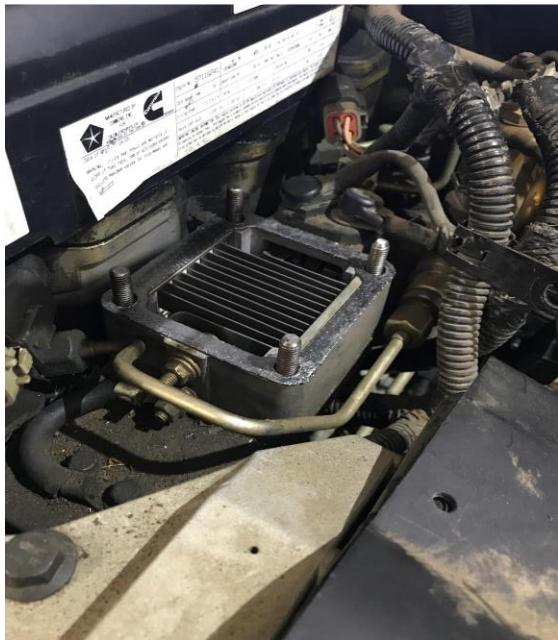
6. Install the Deviant Race Parts intake elbow and firmly tighten the four 13mm nuts provided.
