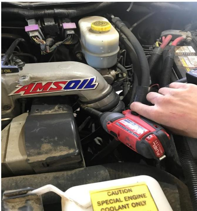
3. Remove the four 10mm bolts holding the factory intake elbow on.
