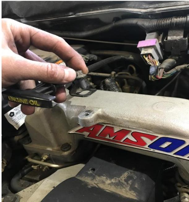
2. Remove the T-Bolt clamp on the intercooler pipe
