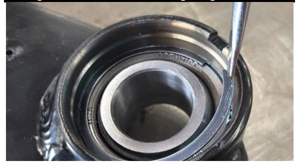
Figure 2: Internal Retaining Ring Removal
