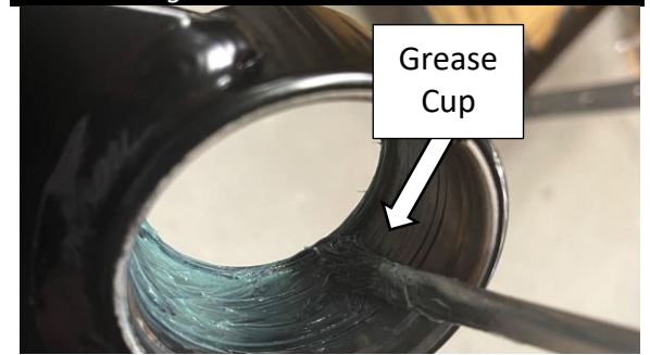
Figure 3: Deburr and Grease
