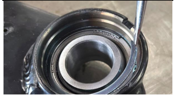
Figure 2: Internal Retaining Ring Removal
