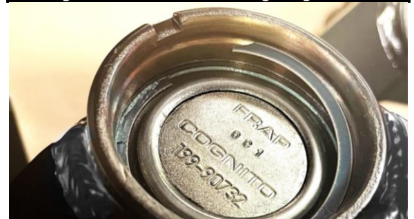
Figure 4: Internal Retaining Ring Install
