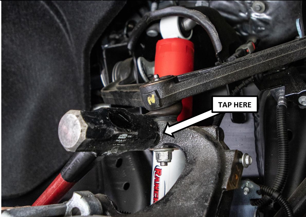
Figure 2: UCA and Spindle Disassembly
