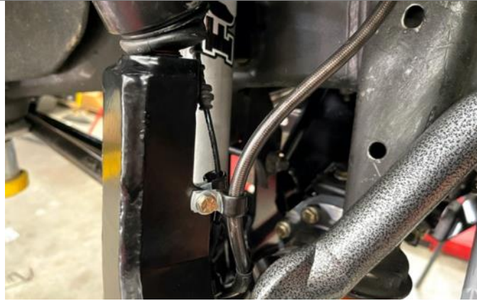
Figure 62: Passenger Side: Top Spindle Tab and P-clamps
