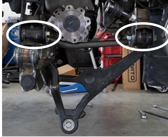
Figure 72: Lower Control Arm Bolts that do NOT get torqued at this step
