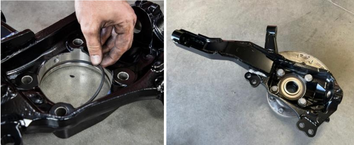
Figure 53: Reassemble Hub Assembly
