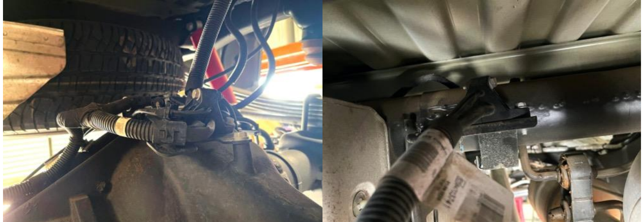
Figure 74: Triangular Bracket Removal
