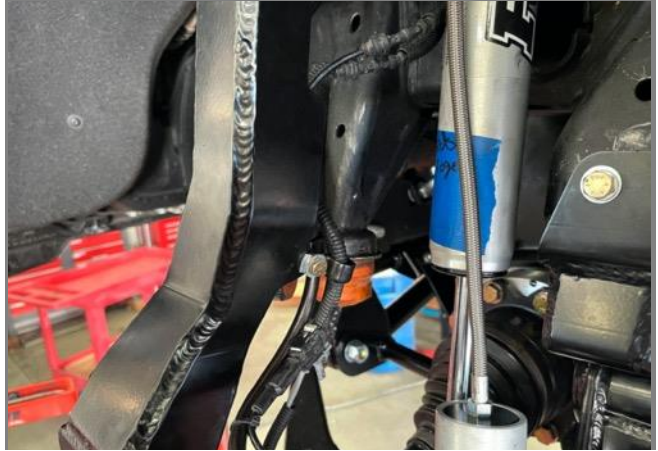
Figure 65: Driver Side Middle Spindle Tab & P-clamps
