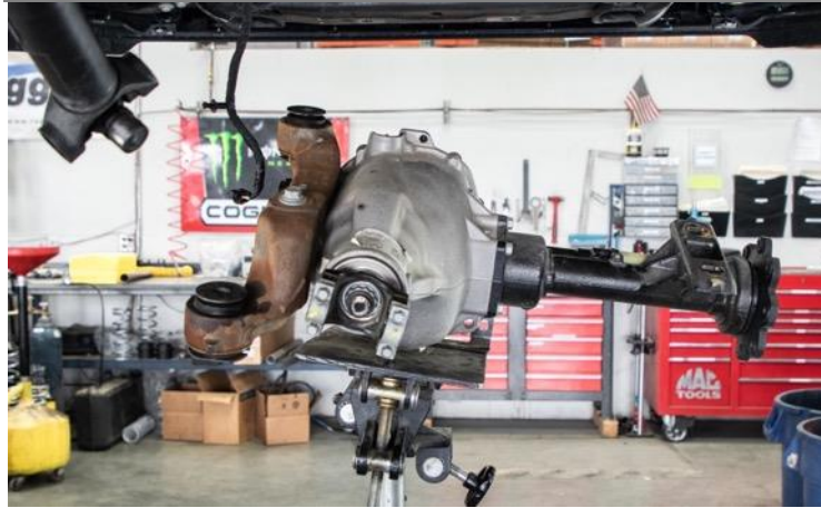
Figure 24: Lower Differential from Vehicle
