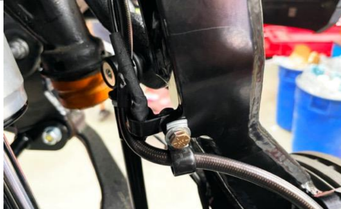
Figure 63: Passenger Side: Middle Spindle Tab and P-clamps
