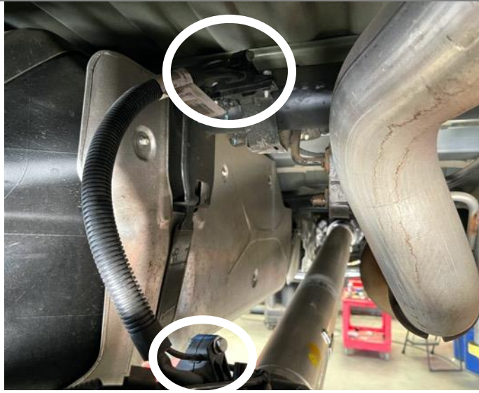
Figure 73: Triangular Plastic Bracket for Rear Brake Harness
