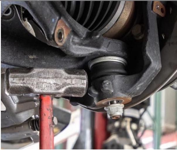
Figure 10: Loosen Lower Ball Joint
