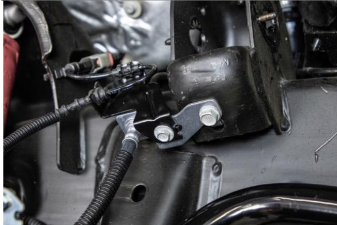
Figure 54: Remove Brake Line Bracket
