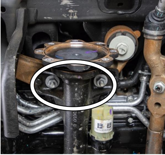
Figure 22: Passenger Side Differential Mounting
