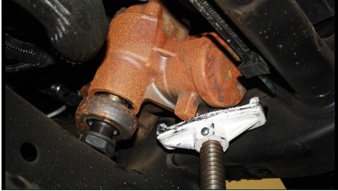
Figure 4: Support the Steering Box with a Jack
