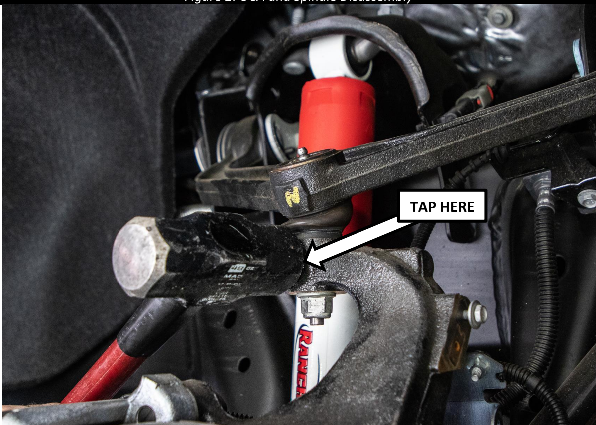
Figure 2: UCA and Spindle Disassembly
