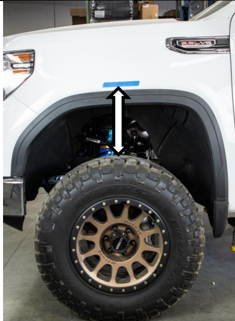
Figure 7: Measuring and Setting Ride Height
