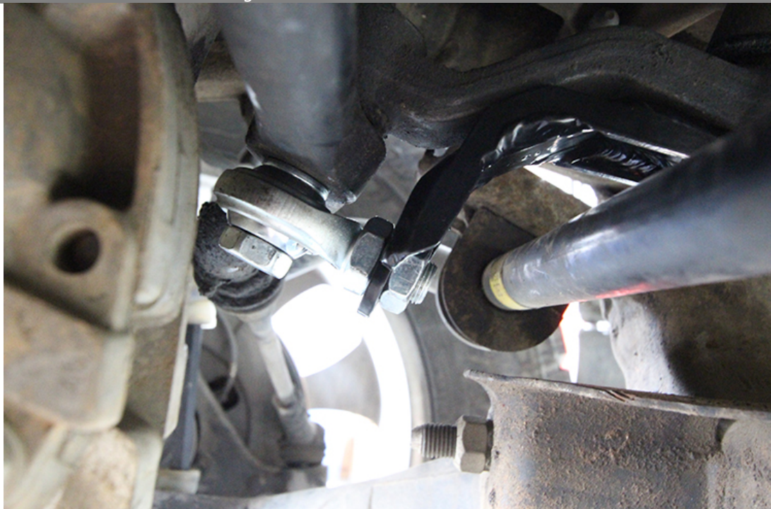
Figure 5: Pitman arm bracket installed
