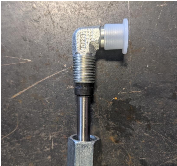
PICTURE 3: CORRECT ALIGNMENT
