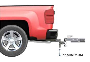
Ensure that you have chosen a hitch that provides enough vertical adjustment to allow your trailers to tow as level as possible while providing enough ground clearance.
