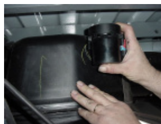
Step 3: Slide fuel valve from bracket.
