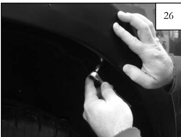
Hold flare in place while you start factory screws using an 8mm socket wrench. Do not tighten.
