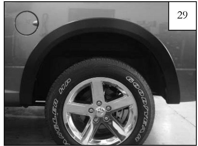
Completed rear flare installation.
