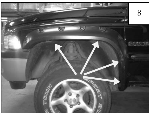
Using a right-angle drill with a #2 Phillips bit, drill four supplied Screws (SW1-0066) through plastic of fender flare and into sheet metal of fender using the indents in the flare as a guide. Install Screws from front to back.
