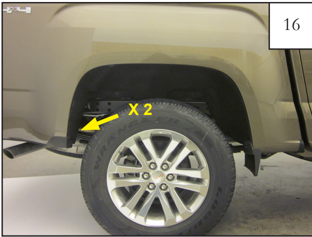
Using a T-15 torx bit, remove two factory fasteners from the mud guard in the lower rear of the wheel well. Discard factory fasteners only.
