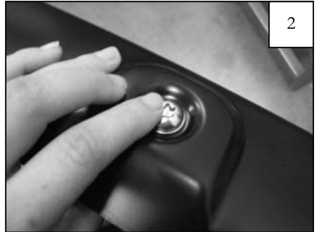
Put each Bolt through a pocket hole in the flare, bolt head on the outside.
