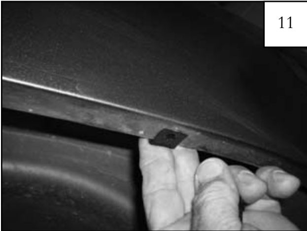
Center a supplied Clip (NU1-0007) over the upper two marks made in Step 9. Clips may need to be adjusted to align with holes in flare. Note: The raised collar on the Clip should face upward into the interior of the fender.
