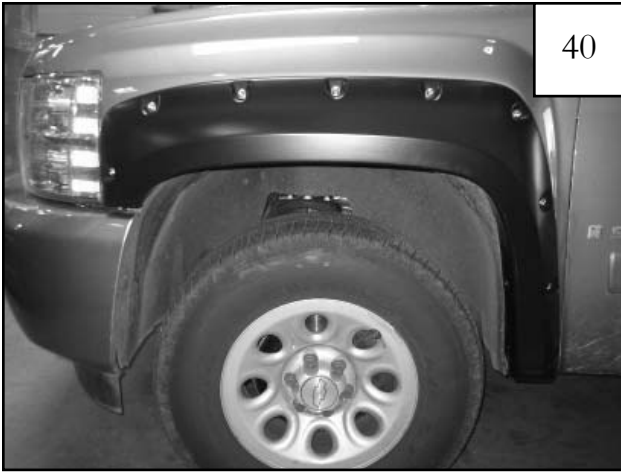
Reinstall wheel. Completed front flare installation.
