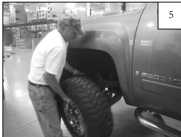
Support vehicle and remove tire.
