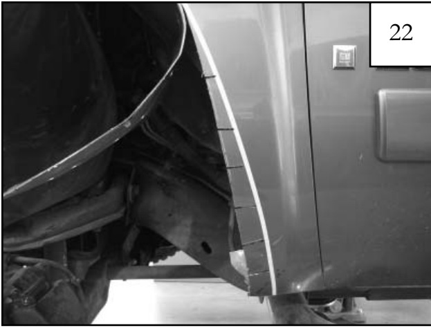
Cut fender approximately every 2" up to edge of masking tape.
