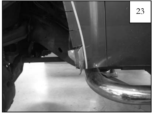
Bend lowest two metal tabs outward.
