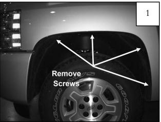
Using a 7mm socket, remove four factory screws. Keep screws for later use.
