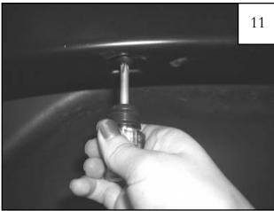
Reposition flare on fender. Start a supplied #14 Truss Head Screw through each topmost hole in the flare, and into each Plastic Clip installed in Step 6.
