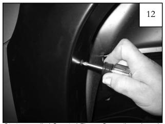
Start a supplied Serrated Flange Screw through each of the remaining holes and into each "S" Clip installed in Step 10. If needed, use awl to locate holes.
