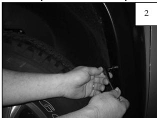
Position flare on fender and reinstall the four factory screws removed in Step 1, be sure to not tighten.
