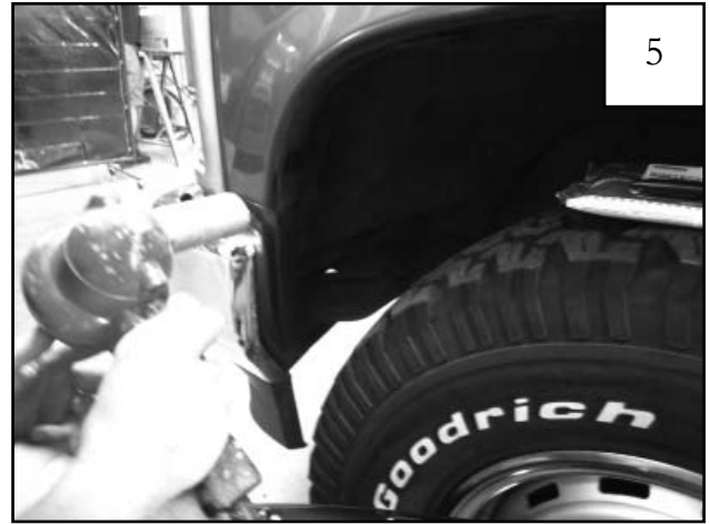
Use hair dryer or heat gun to heat molding. This helps loosen the adhesive making it easier to remove.
