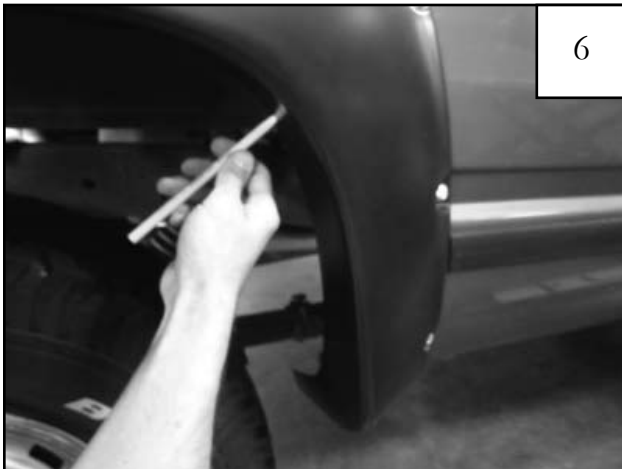
Hold flare in position on fender using moderate pressure. Using a grease pencil, mark five hole locations using the holes in the flare as a guide. (See Step 7)
