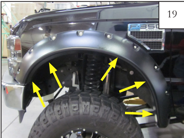
Install flare using factory screws removed in Step 16 through holes indicated.
