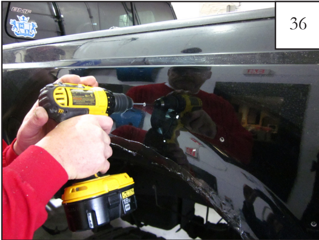
36 Using a 1/8" bit, drill marked hole locations. Then, using a 13/64" bit, drill holes again.
