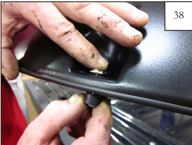
38 Thread bolt (SW1-0045) through pocket hole in flare then install spacer (SP1-0009) over end of bolt. Hand tighten spacer on bolt until snug near flare plastic. For rear mounting bolt use (SW1-0056) and space (SP1-0009).
