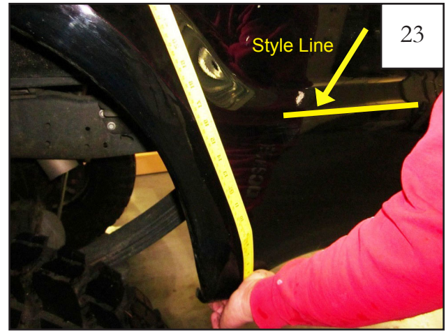
Starting from bottom under edge below mark made in previous step, measure up following curve of wheel well approximately 15" to lower style line and mark with grease pencil.
