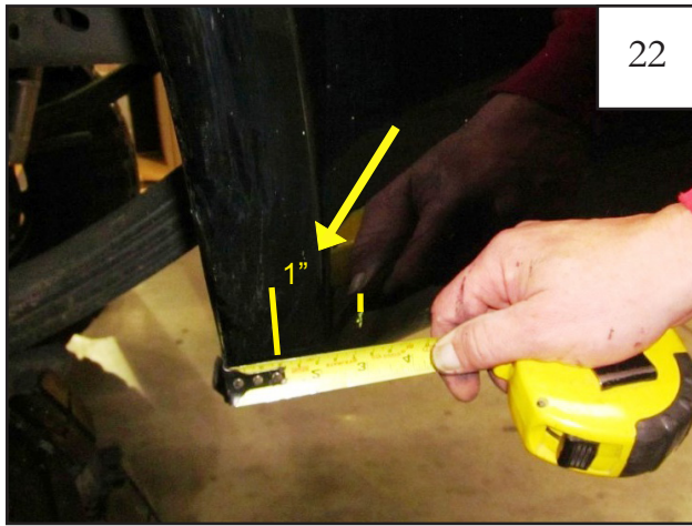
Measure 1" from back side of rear wheel well and front wheel well and mark using a grease pencil.
