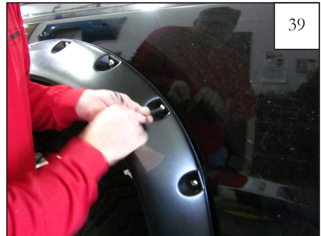
39 Reattach factory support bar bolt, removed in Step 37, through front mounting hole. Using torx bit (SW1-0052), start bolts installed in Step 38 through holes drilled in Step 36. Once all bolts are in place, tighten all screws.
