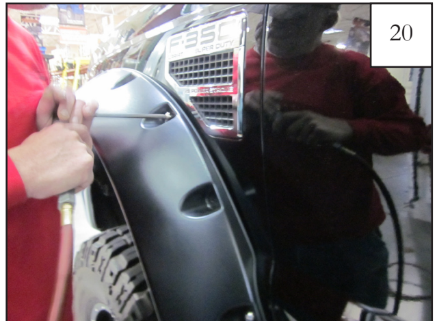
Using torx bit (SW1-0052), start bolts installed in Step 18 through holes drilled in Step 17. Once all bolts are in place, tighten all screws.
