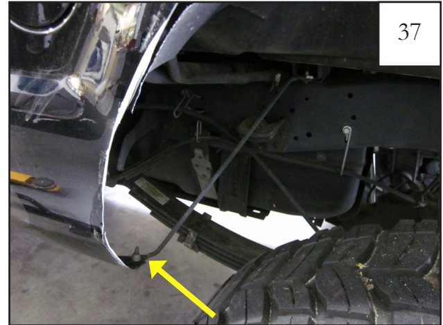
37 Remove factory support bar bolt, and save for reinstallation.
