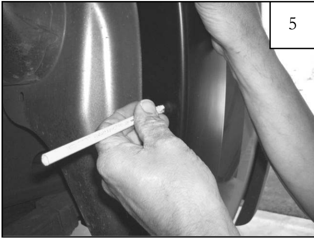
Holding flare in position on fender, use a grease pencil to mark five clip locations. See step 6.
