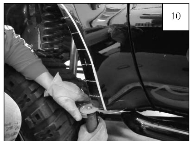
Using a cut-off wheel, cut fender along marked lines up to inner edge of tape.
