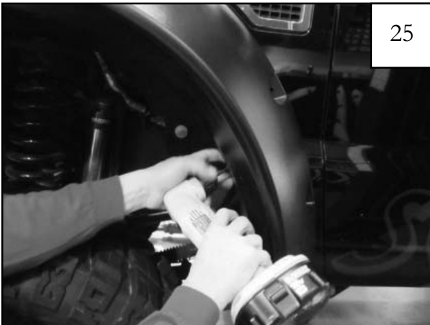
Install screw (SW1-0056) into holes drilled in previous step. Tighten ALL screws installed in Steps 23 & 24 to ensure proper alignment of flare for pocket hardware installation.
