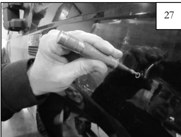
Remove screws and flare. Using marks made with scratch awl as a guide, use a center punch to score sheet metal prior to drilling.
