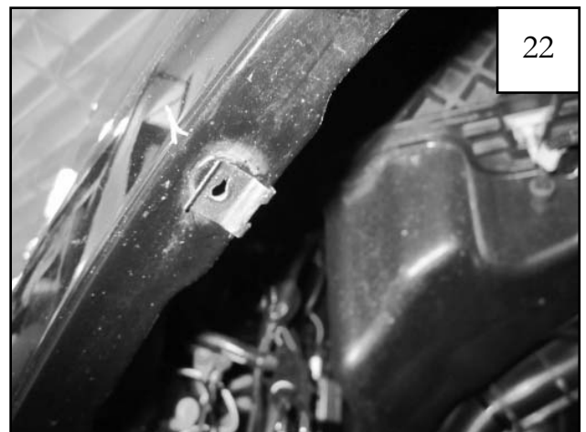
Install Clip (CL1-0022) over hole on outer edge where indicated in Step 21.
