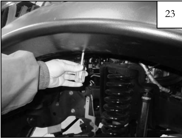
Install flare and start Screw (SW1-0056) through clips installed in previous step with a #2 Phillips Driver. Do not tighten.
