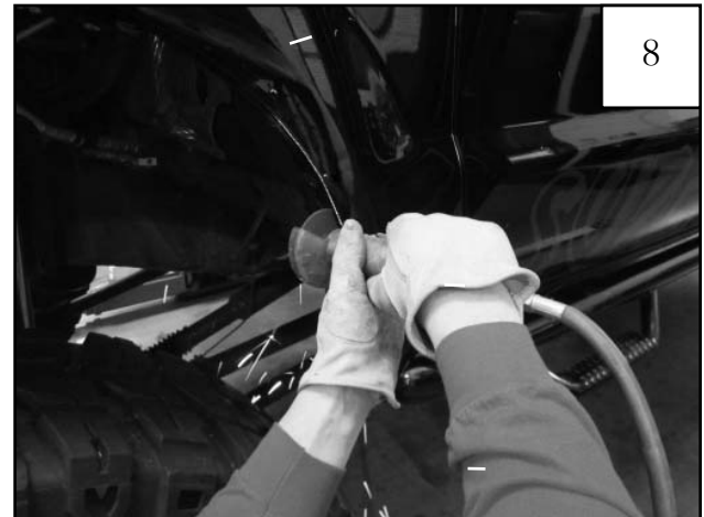
Using a cut-off wheel, cut and remove inner flange.
