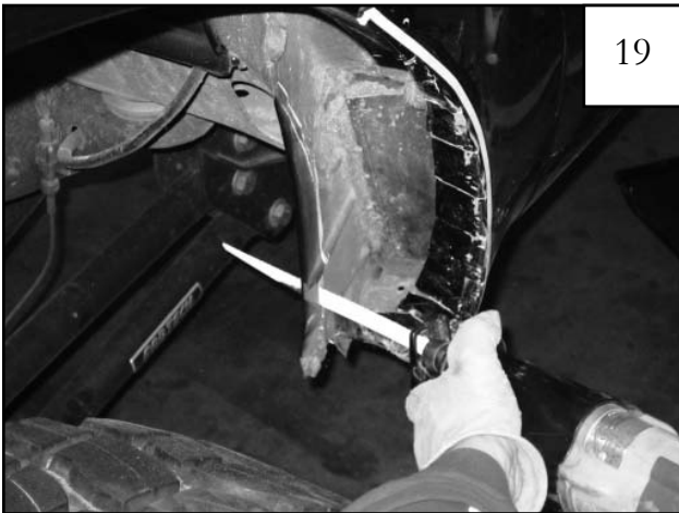
Using a Sawsall, cut along reference line.
