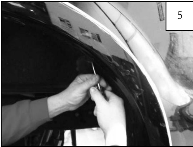
Using a pry tool, remove two factory installed tuflocs from splash guard
