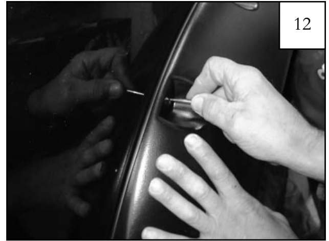
With a partner holding flare in place, using a scratch awl and pocket holes in flare as a guide, mark vehicle for drilling.
