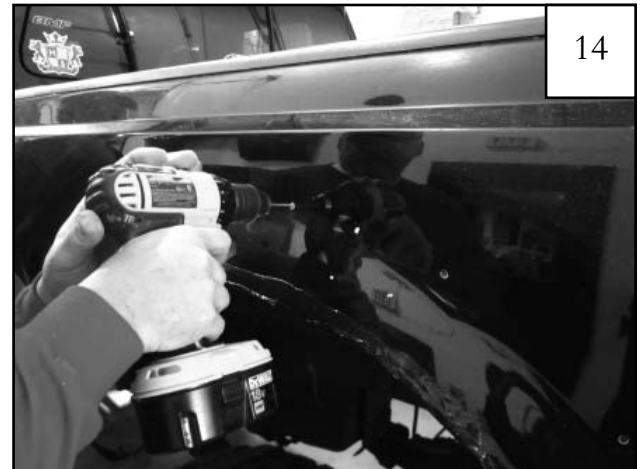
Using a 1/8" bit, drill marked hole locations. Then, using a 13/64" bit, drill holes again.
