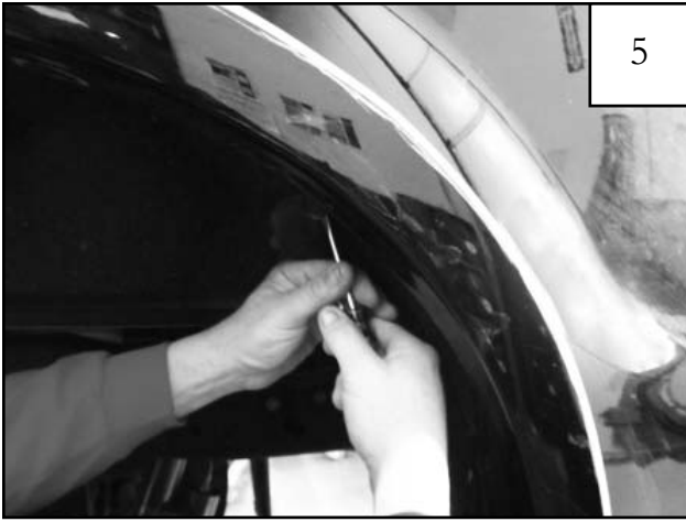
Using a pry tool, remove two factory installed tuftlocs from splash guard
