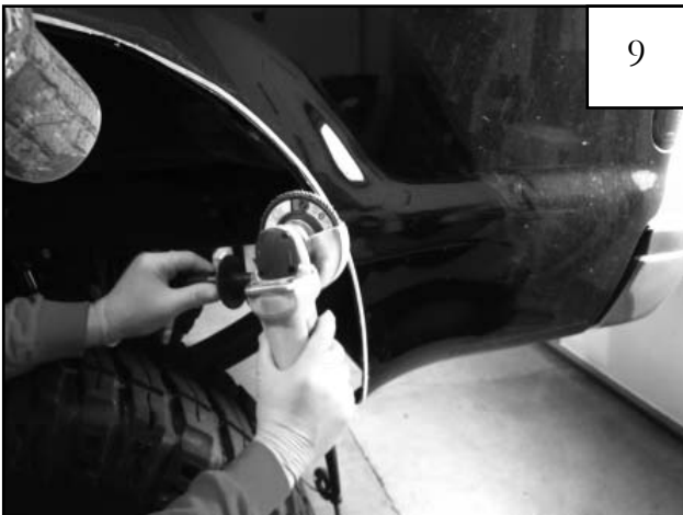
Using a grinder, deburr cut edges.
