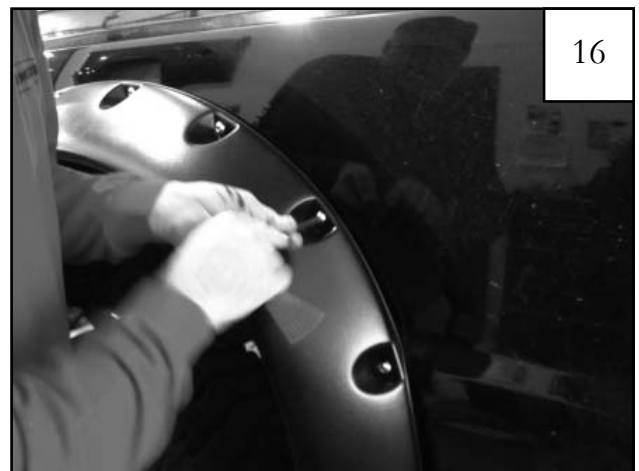
Using torx bit (SW1-0052), start bolts installed in Step 15 through holes drilled in Step 14. Once all bolts are in place, tighten all screws.
