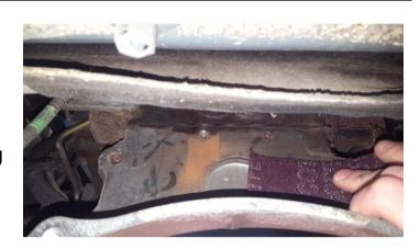
3. Make sure the M8 and M12 bolts can be threaded in by hand. You may need to run a thread chaser down the bolt holes or use penetrating fluid.
