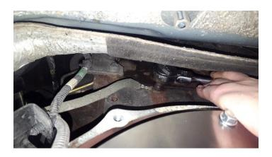
2. Use an abrasive pad to remove all rust and debris. The plate must sit flush to the motor.
