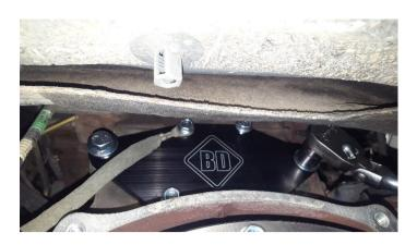
If your truck has a TCC crossover tube, DO NOT try to slip the plate between the tube and the block, this may cut the O-ring.
