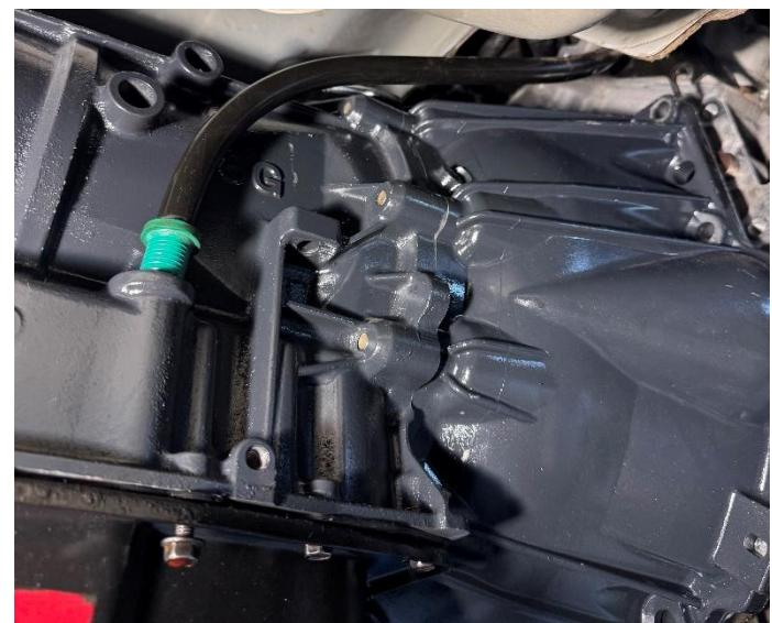
Slide the transmission onto dowel pins. The torque converter must rotate freely by hand. Ensure the transmission is seated as well as possible and align the bolt holes between the flywheel and the torque converter before threading in any bolts.
