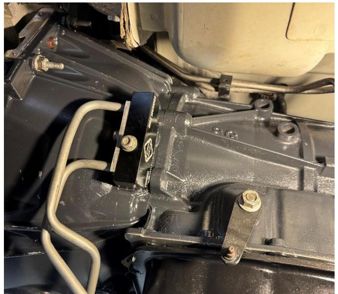
Push in the transmission electrical connector with the black tab facing up and turn clockwise.
