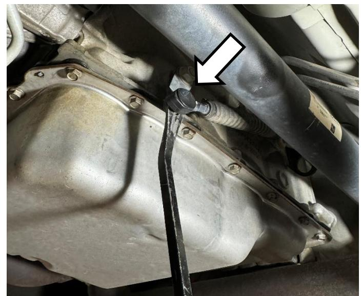
Remove the **2 x T50 torx bolts** that hold on the range selector bracket.
