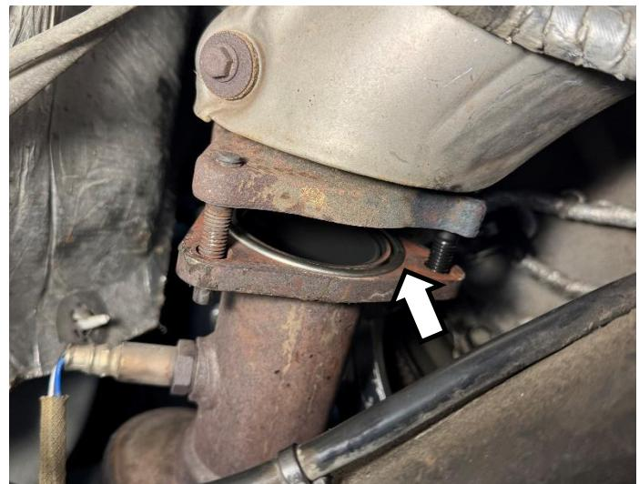
Install **3 x nuts** on both sides of the exhaust using a **15 mm socket**.
