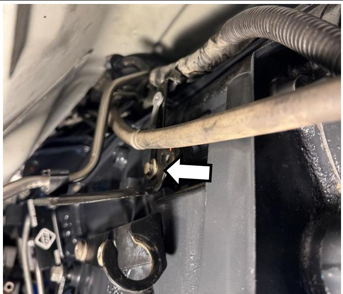
Install the **1 x bolt** that holds on the cooler bypass block using a **13 mm socket**.
