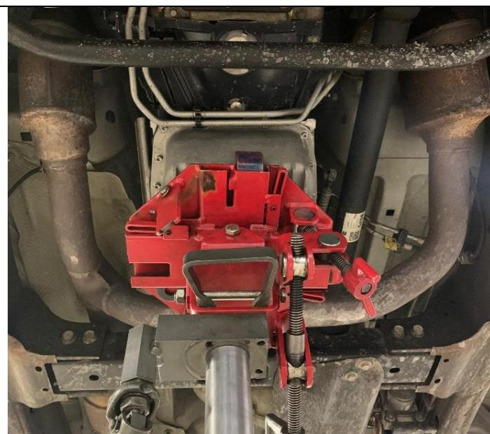
Remove the **2 x nuts** in the center hole of the cross member and remove cross member using a **15 mm socket**.
