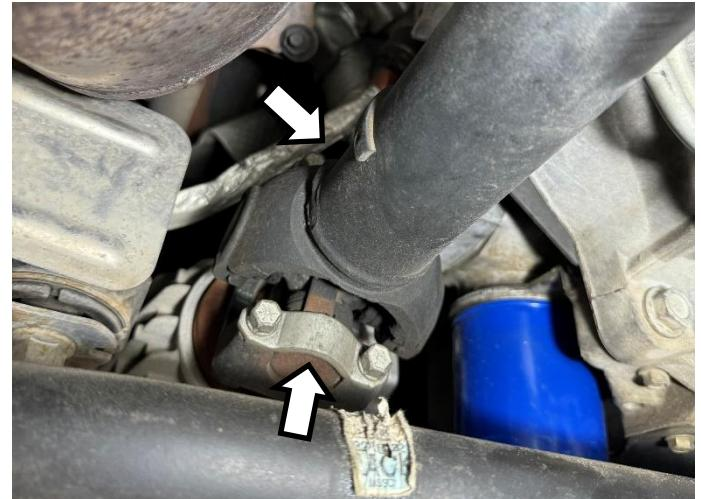
Remove the front driveshaft by pushing the driveshaft into the transfer case to allow room to remove the pinion from the yoke.
