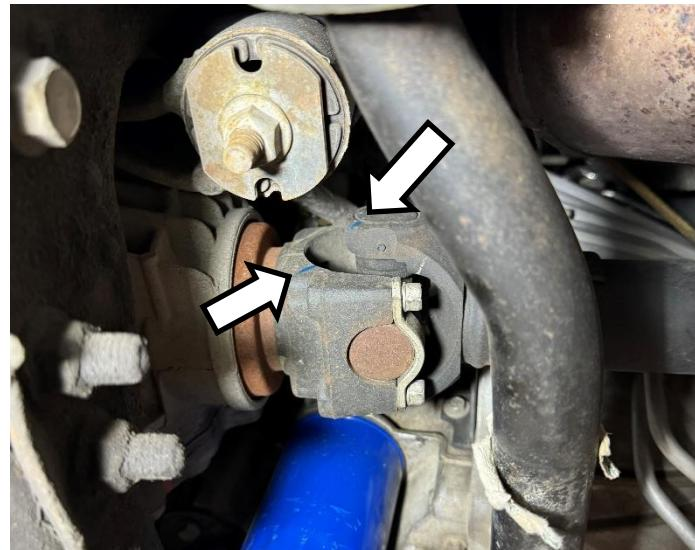
Remove the **4 x bolts** that hold on the yoke retainer using an **11 mm socket**.
