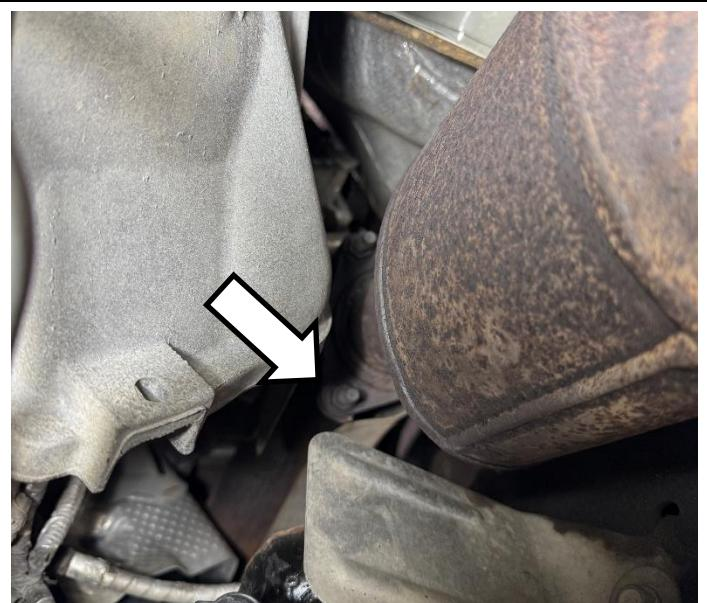
Remove the **1 x bolt** that clamps the front ball flange to the rear section using a **15 mm socket** and remove.
