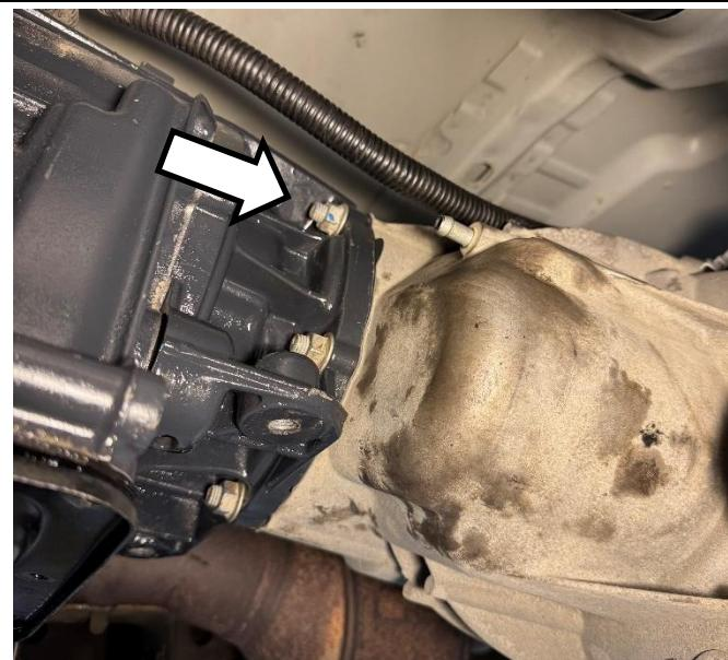
Install all three electrical connectors into back of transfer case.
