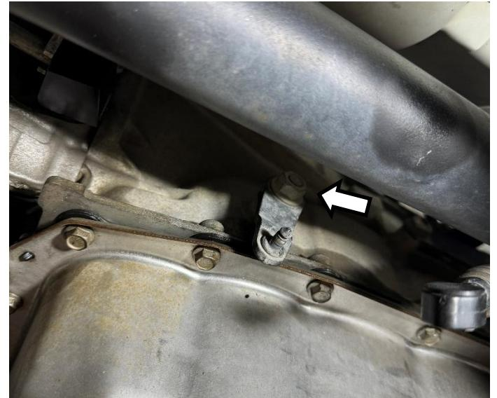
Remove the **1 x bolt** that secures the fuel line bracket to the transmission using a **13 mm socket**. Reposition the bracket.
