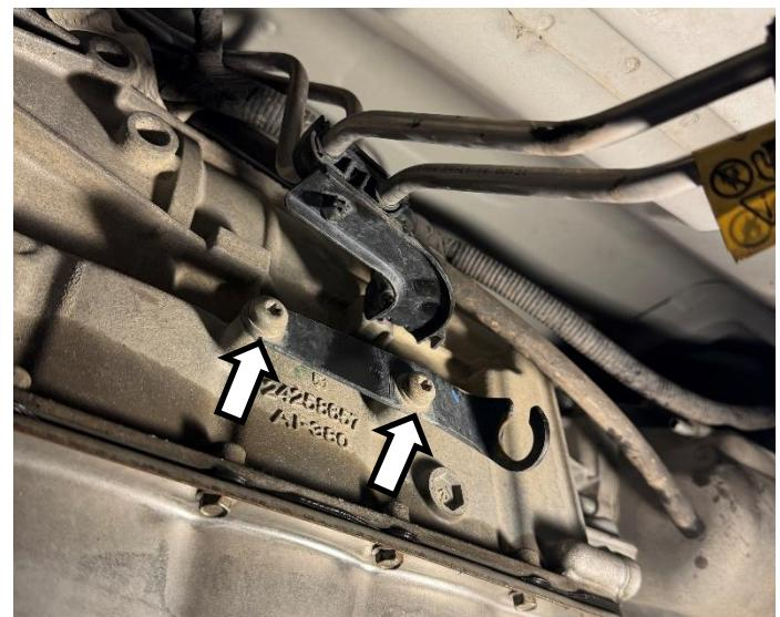
Remove the **1 x nut** that holds on the range selector lever using a **13 mm socket**.
