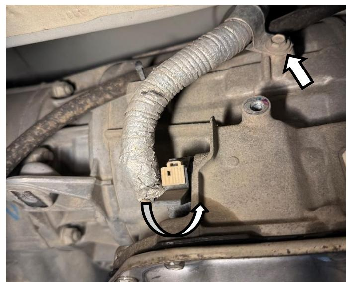
On the range selector cable push up on the end of the clip to remove.
