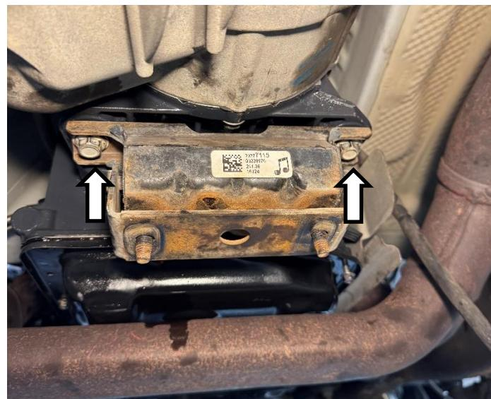
Install the transmission cross member with the **4 x bolts and nuts** on the outside using a **21 mm socket** and the **2 x nuts** that screw onto the transmission mount studs using a **15 mm socket**.
