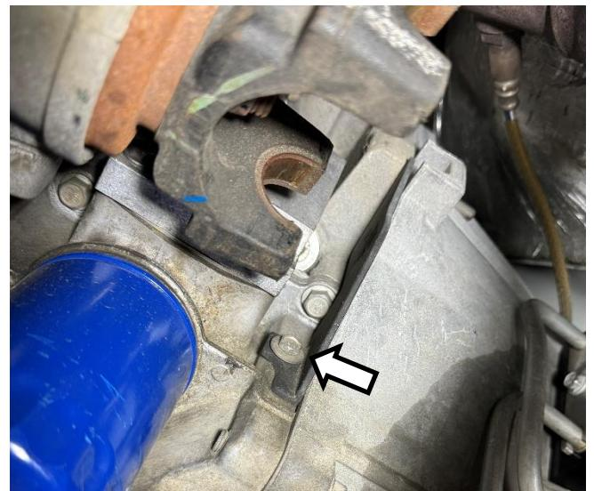
If the vehicle is equipped with a front drive shaft, install the slip yoke on the front driveshaft into the front of the transfer case.
