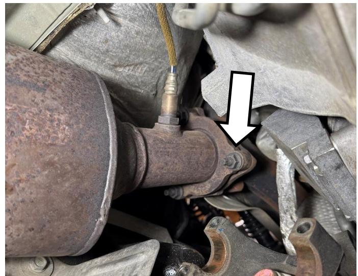
Connect front of exhaust to rear section with the ball flange and install **1 x bolt** using a **13 mm socket**.
