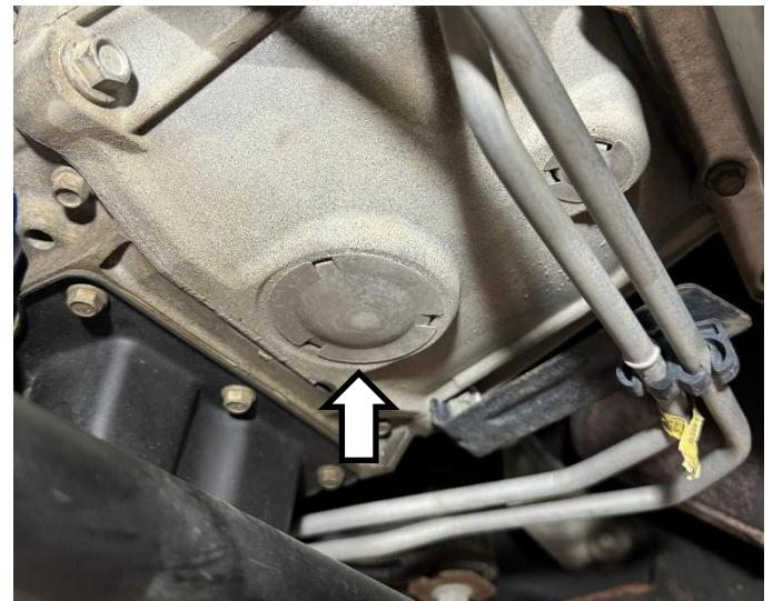
Remove the **1 x bolt** that holds on the left flywheel inspection cover using a **10 mm socket** and remove cover.
