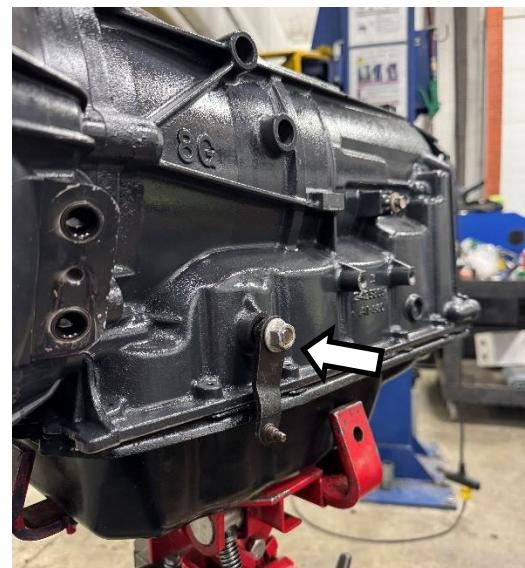
Install the range selector bracket from the old transmission onto the new transmission.
