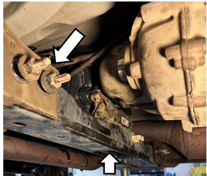
From the torque converter access hole, push the torque converter forward through the access hole to seat the converter pilot into the crank bore.
