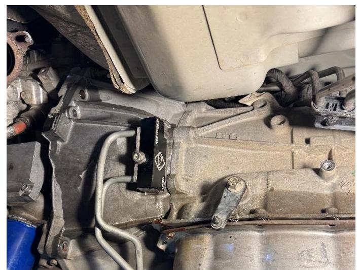
On the passenger's side of the transmission remove the 1 x bolt that holds the cooler line bracket to the bellhousing using a 15 mm socket.
