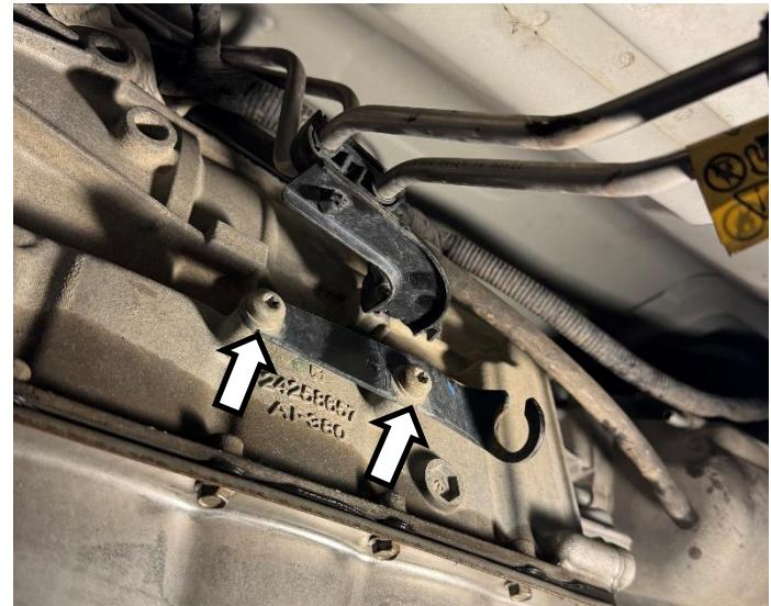
With transmission well supported, raise transmission up to back of engine while simultaneously installing the transmission dipstick tube with the new seal provided.
