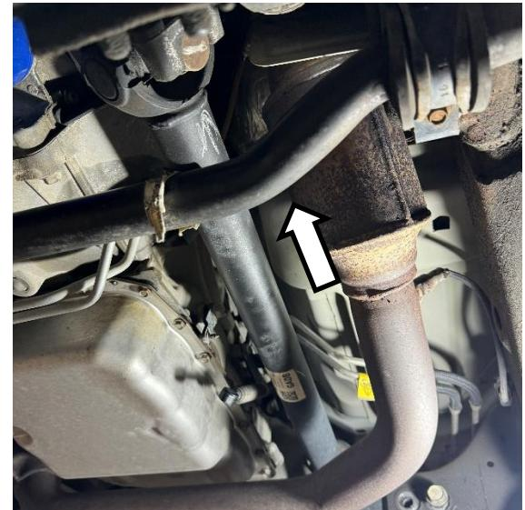
On the rear driveshaft, mark the relationship of the driveshaft to the front axle pinion yoke.
