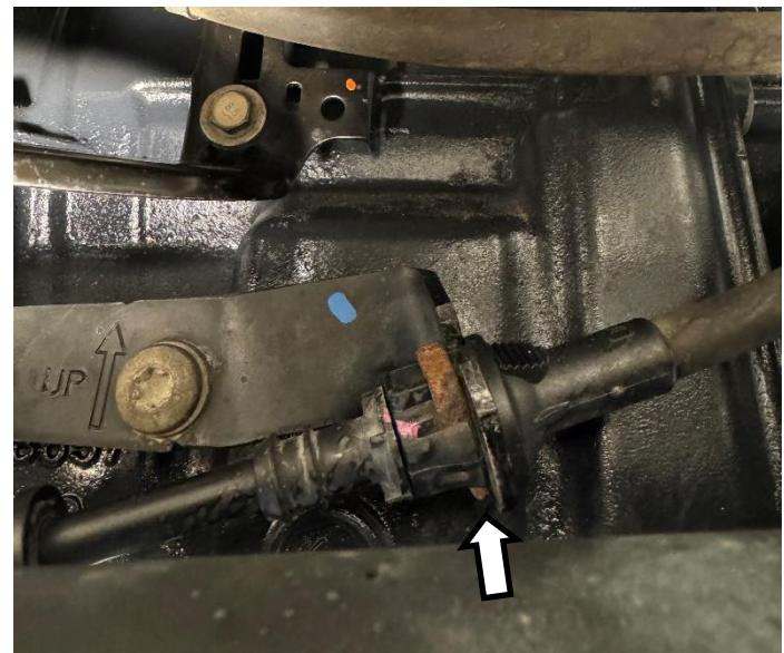
Use a pry bar or flat head screwdriver to pop off the front of the range selector cable.
