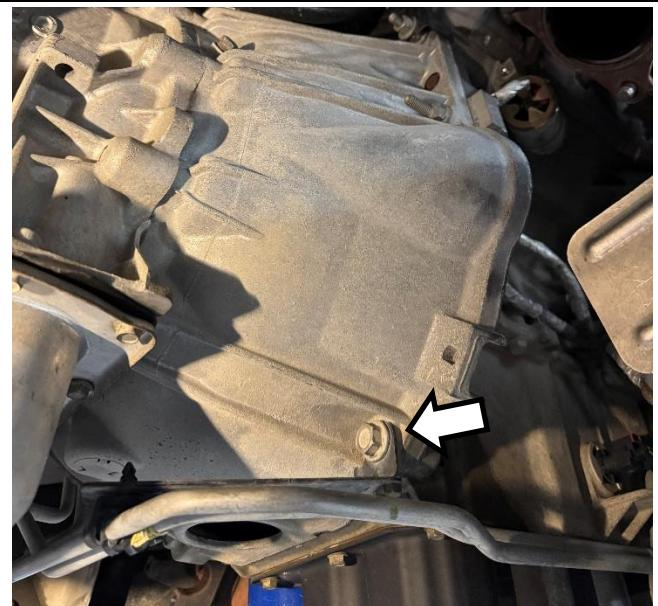
On the passenger's side of the transmission, remove the 1 x nut that is holding on the transmission dipstick bracket using a 13 mm socket.
