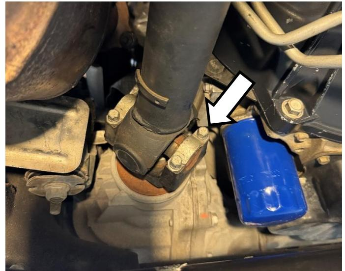
Install slip yoke of rear driveshaft into the back of the transfer case.
