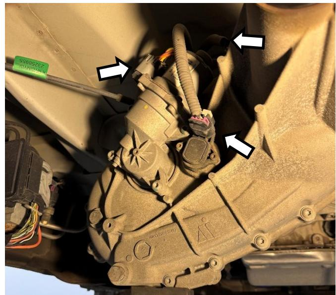
Remove the transmission vent tube retaining nut on the back of the transmission and reposition the vent tube bracket.
