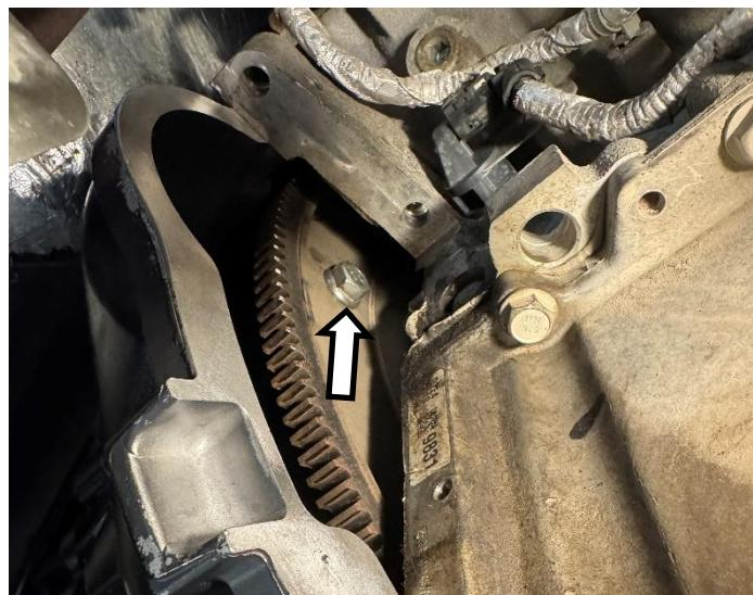
Install the flywheel inspection cover on the passenger's side with **1 x bolt** using a **10 mm socket**.
