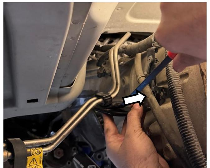
Remove the **1 x bolt** that holds on the cooler bypass block on the driver's side of the transmission using a **13 mm socket**.
