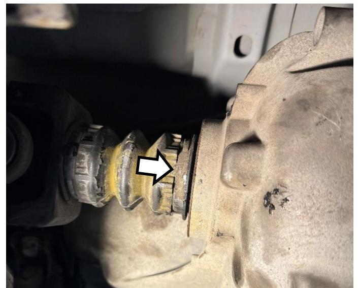
Align the reference marks made during removal and install the 2 yoke retainers and **4 x bolts** using a **11 mm socket**.
