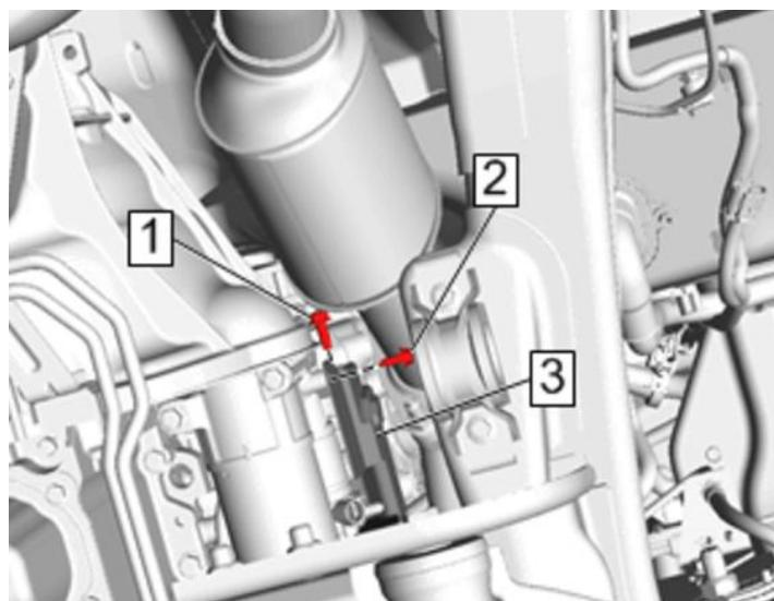
Install the torque converter access plug.
