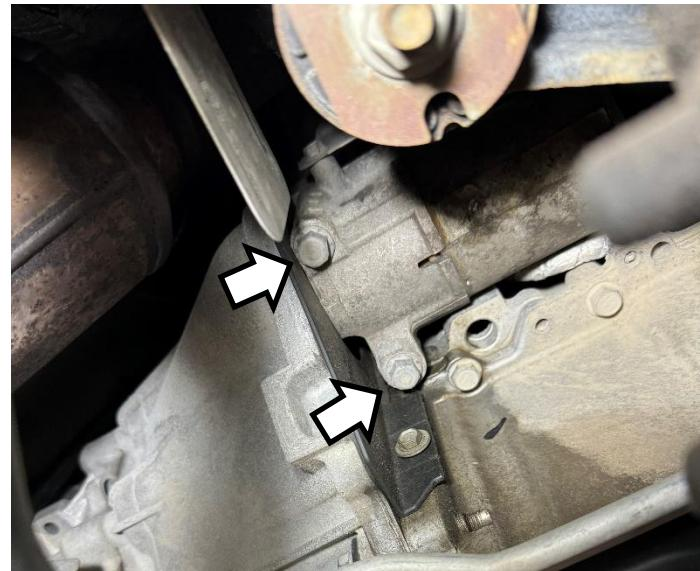
Remove the **1 x bolt** that holds on the flywheel inspection cover using a **10 mm socket** and remove cover.
