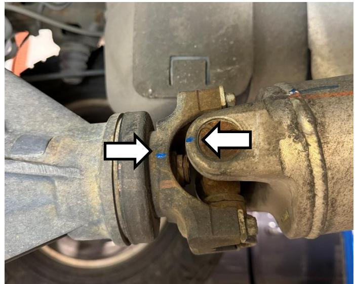
Remove the **4 x bolts** that hold on the yoke retainer using an **11 mm socket**.
