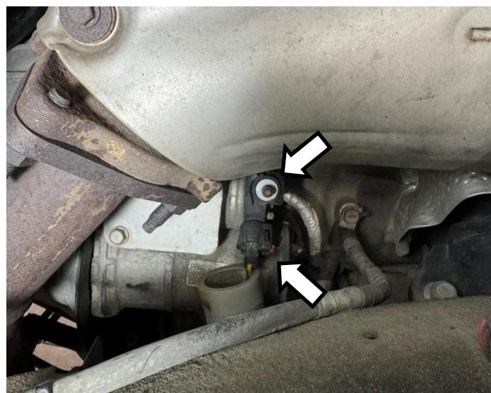
Remove the starter heat shield by taking off the 1 x bolt on the side of the bracket using a 13 mm socket and the 1 x bolt on the top of the bracket using a 10 mm socket.
