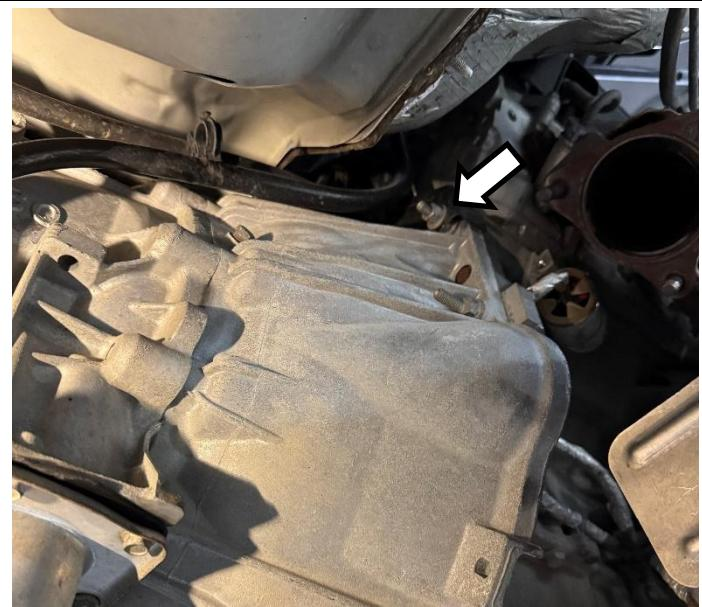
Remove the remaining 7 x bolts that hold on the transmission to the back of the engine using a 15 mm socket while simultaneously pulling out the dipstick tube on the passenger's side.
