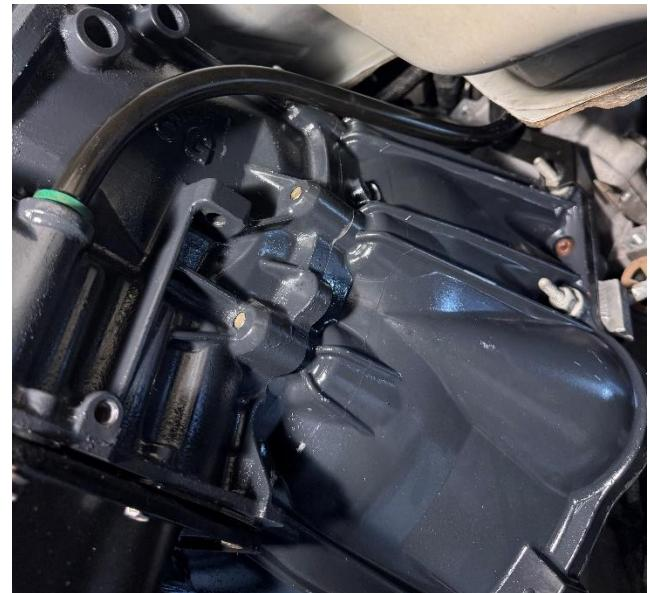
Attach the transmission vent tube to the port on the top of the transmission.
