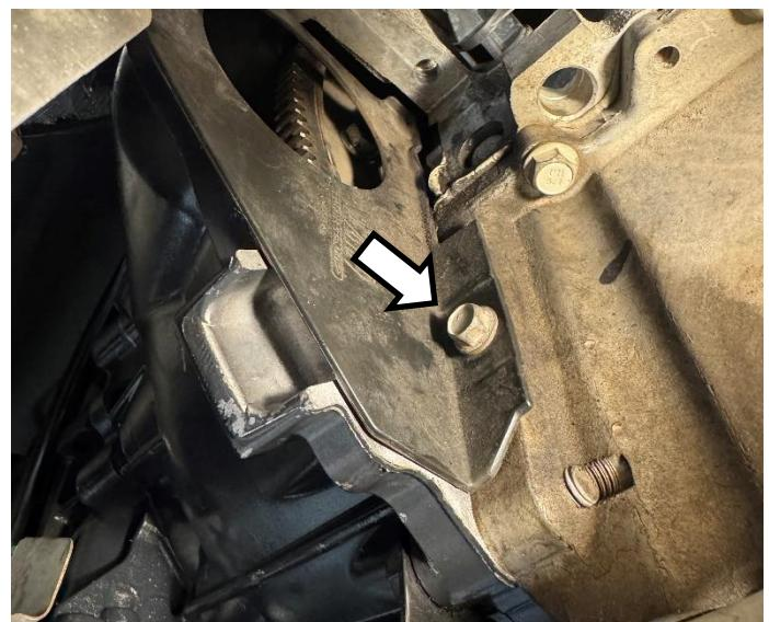
Remove the 8 bolts that hold on the steering gear skid shield and remove.
