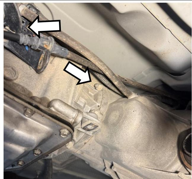
Disconnect all O2 electrical connectors from the front of the exhaust. There are 2 sensors per side.
