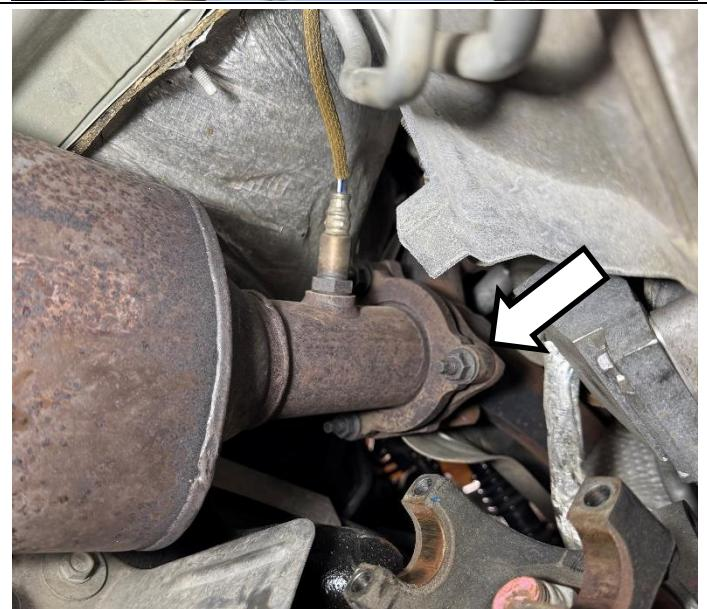
Remove the **3 x nuts** that hold the collector to the manifold on the passenger's side using a **15 mm socket**.
