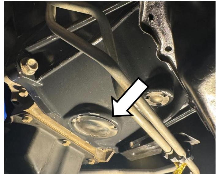
Install the flywheel inspection cover and **1 x bolt** using a **10 mm socket**.
