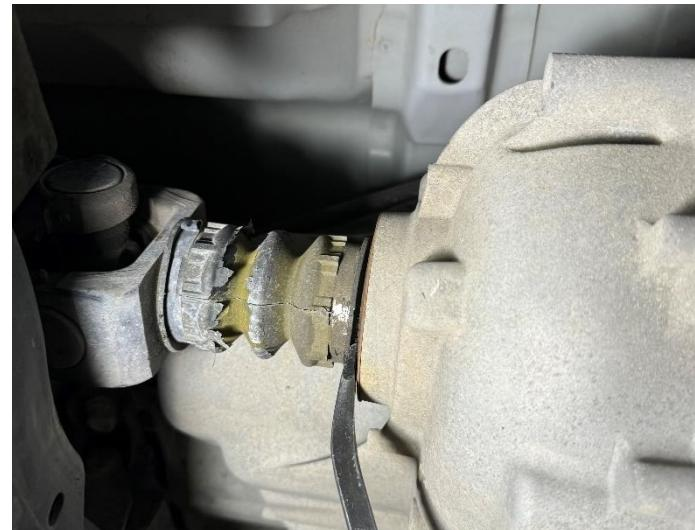
On the front driveshaft, mark the relationship of the driveshaft to the front axle pinion yoke.
