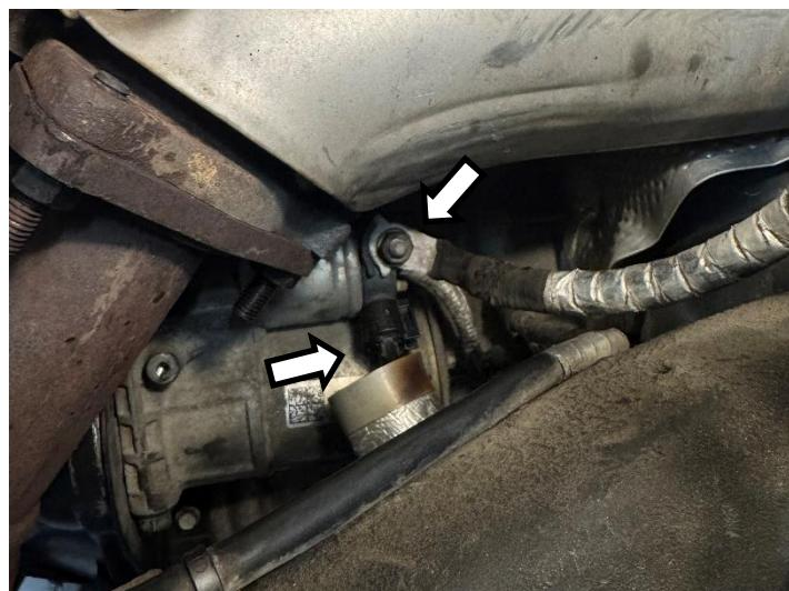
Install the **2 bolts** that hold on the starter heat shield.
