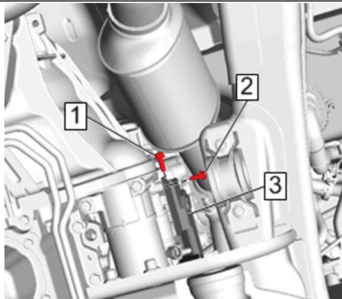
**Warning:** Complete this step carefully as the starter will fall after removing bolts.
