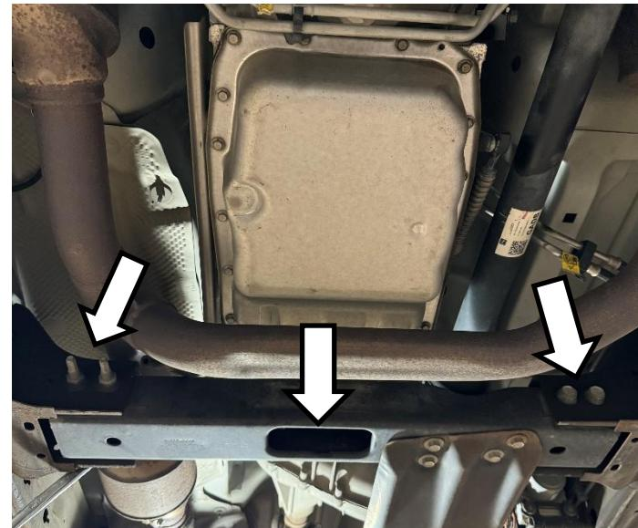
Remove the **2 x bolts** that hold on the transmission mount using a **15 mm socket** and remove.
