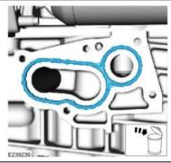
37. Install oil filter adapter and the bolts and stud bolt. Tighten to 12 Nm (106 in-lb)
