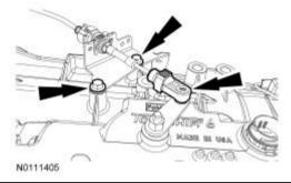
29. Install the transmission vehicle harness connector and lock the transmission vehicle harness connector by rotating the outer shell clockwise.
