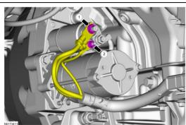
35. Install the starter motor cable cap.
