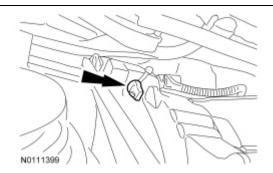
28. Position the selector lever cable bracket and install the 2 bolts. Tighten to 48 Nm (35 ft-lb).
