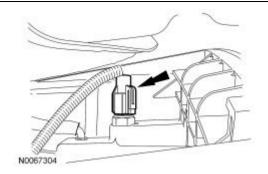
27. For vehicle with electric shift transfer case; disconnect the gearmotor encoder connector and the gearmotor electrical connector.
