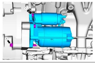
Remove the retainers and remove the starter dust shield.
