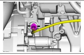
32. Secure the wiring harness and tighten to 12 Nm (106 in-lb).
