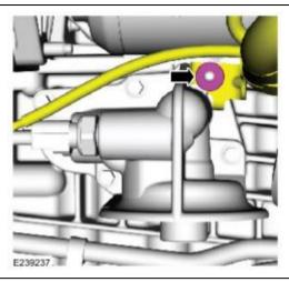
6. Remove the stud bolt, the bolts and the oil filter adapter.
