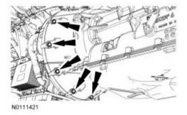
5. Install 6 new torque converter nuts. Tighten to 48 Nm (35 ft-lb).
