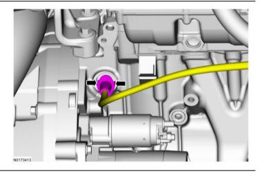
13. Remove the 3 bolts securing the starter and remove the starter.
