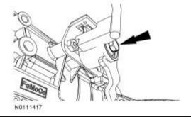
19. Tighten the transfer case linkage bracket bolt to 115 Nm (85 ft-lb).
