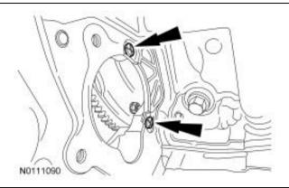
15. Remove and discard the 6 torque converter nuts.
