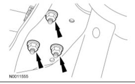
26. Install RH engine support insulator nuts. Tighten to 115 Nm (85 ft-lb).
