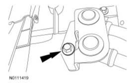
34. Remove the lowers transmission fluid filler tube bolt and position and transmission fluid filler tube aside. Remove and discard the transmission fluid filler tube Oring.
