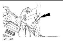
25. Remove the bolt and transfer case linkage bracket.
