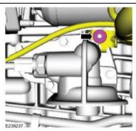
39. Connect the oil temperature sensor and oil pressure switch electrical connectors.
