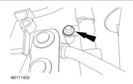
35. Remove the 11 bolts and remove the transmission from the engine dowel pins.
