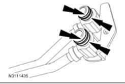
10. Position the transmission fluid cooler tubes in the transmission case and install the bolt. Tighten to 25 Nm (18 ft-lb).
