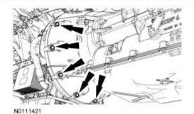
36. Slide the transmission back enough to install the Torque Converter Retainer and remove the transmission.
