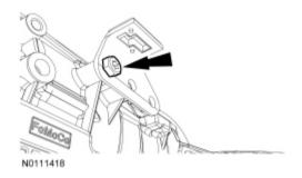
26. Disconnect the 3-position mode switch electrical connector.
