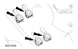
20. Remove the 3 LH engine support insulator nuts.
