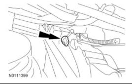
19. Remove the 4 RH engine support insulator nuts.
