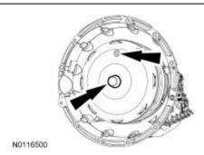
3. Install the Torque Converter
