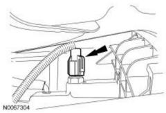
Position the transfer case linkage bracket and loosely install the bolt.
