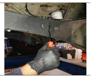
Remove the lower mounting bolts on the shock absorber from both sides of the vehicle. (18mm socket) then move the bottom of the shock out of the mount.
