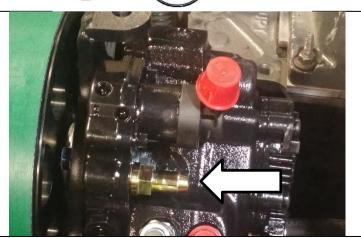
Install -6 JIC fitting (PN 1500416) into the return port of the CP3 as shown. Using supplied seal washer (PN 1502019).
