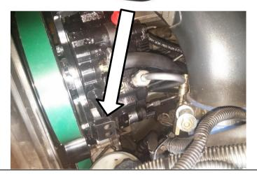
Install supplied upper radiator hose using the factory clamps.
