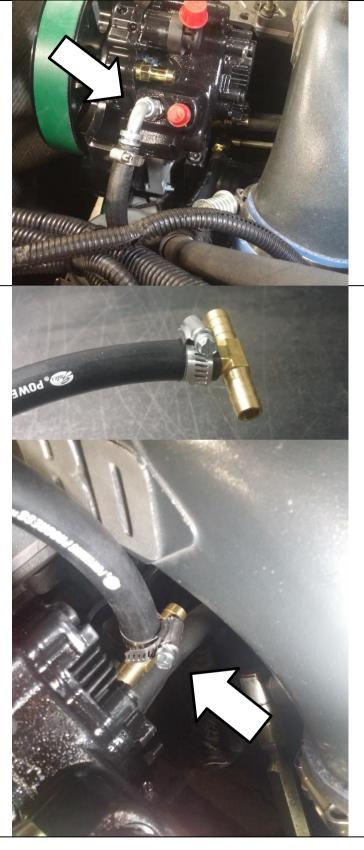
Insert  $\frac{1}{2}$ " tee into the  $\frac{1}{2}$ " fuel hose supplied using a gear clamp.
