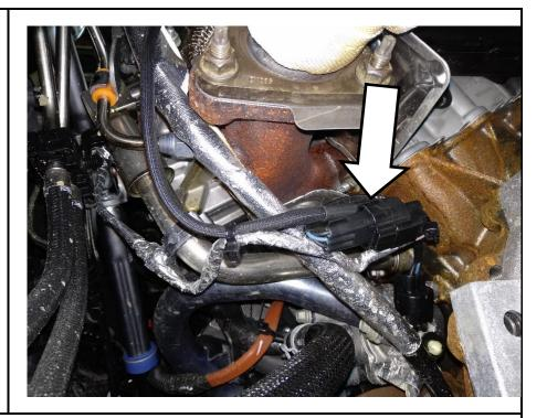
It is necessary to remove the rear belly pan to access the crankshaft position sensor.
