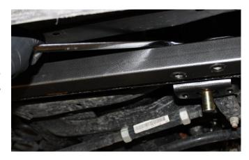
Install two bolts through the small holes in bearing mounting area, so that the threads are hanging through the bracket.
