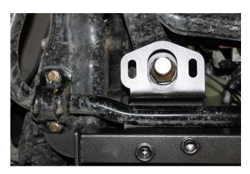
NOTE: 1032003 Kits - Center the SBS bracket on the sector shaft using the slots provided. Tighten both 5/8" bolts using a 15/16" wrench (112 lbs-ft).
