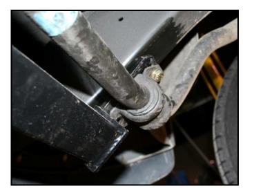
It may be necessary to loosen the sway bar end link bolts to ease installation. (15mm)
