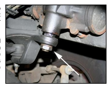
A 1-1/4" deep socket (180 lbs-ft) should be used to install the new sector shaft nut (1302010), re-using the stock lock washer.
