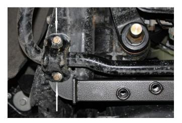
NOTE: 1032003 Kits - Use the 2x 5/8" bolts and washers to center the SBS bracket on the SBS bar.
