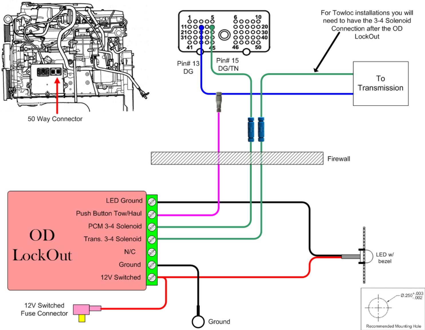
**Note: When using OD Lockout unit with a BD TowLoc, the 3-4 solenoid connection must be made after the OD LockOut connection.**
