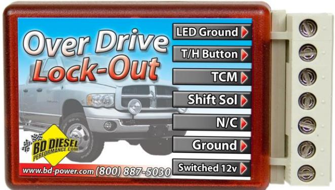
You will need to locate a clean ground point for the module. Underneath the steering column you can utilize a grounded mounting bolt for this purpose. Connect the grounded BLACK wire to the “Ground” input of the module.
