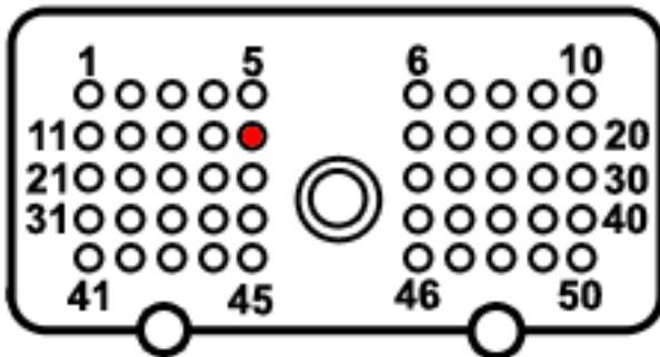
Cut this wire and attach a Posi-Lock on both sides of the cut wire. Attach the BLUE wire to the posi-lok connection closest to the PCM. Also attach the VIOLET wire to the posi-lok connection traveling towards the transmission.
