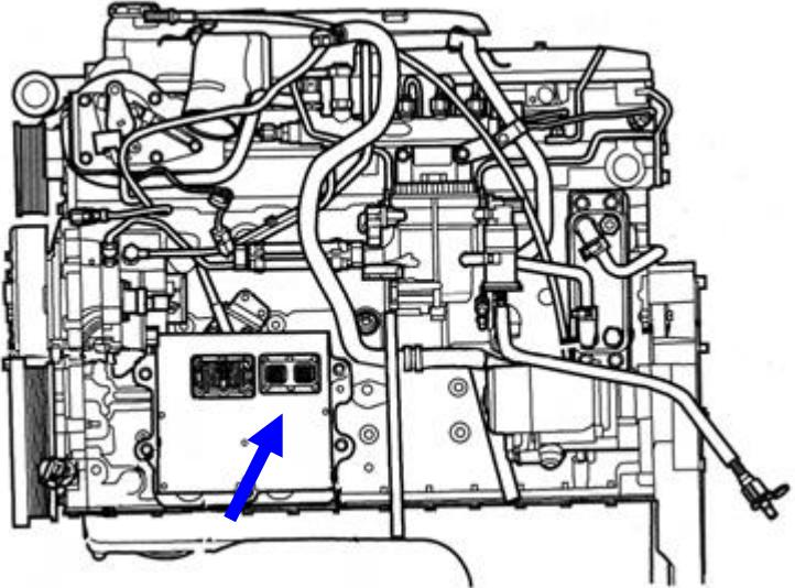
Find **pin# 15** on the 50-way PCM connector - It will be a Dark Green with a Tan tracer wire.
