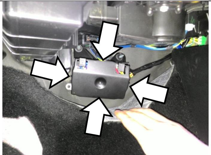
Disconnect the blue connector on the control module.
