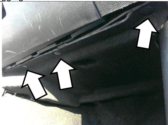
Disconnect the small wire for the under dash LED by pushing in on the tab to release it. Move this panel out of the way.
