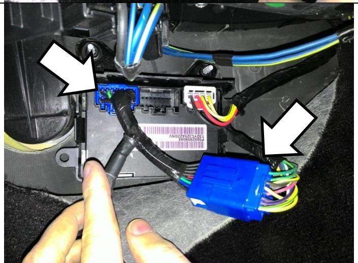
Install the two supplied relays into the BD wiring harness.
