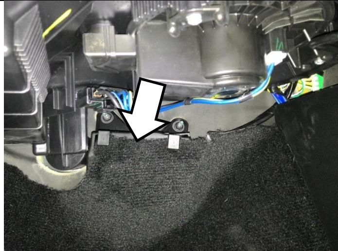
Unclip the plastic cover to expose the drivetrain control module. (4 clips)
