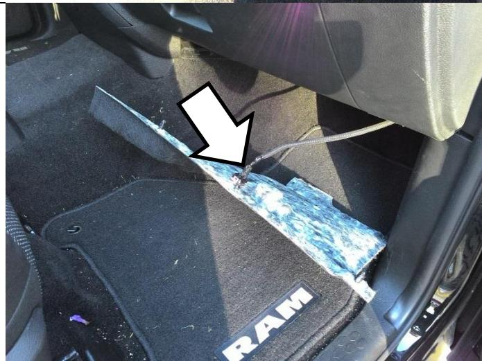
Pull the carpet back to expose the plastic cover protecting the drivetrain control module.
