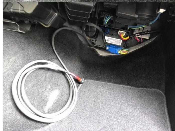
Locate a spot to mount the switch. This may be below the 4wd switch or left to the drivers preference.
