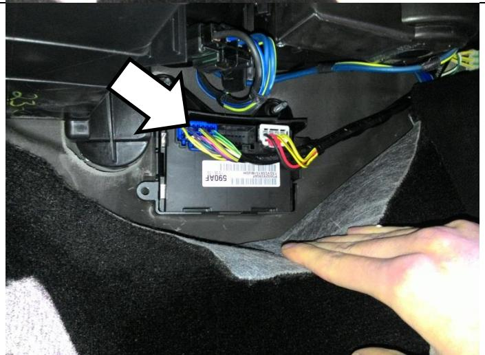
Plug the supplied BD harness into the control module and connect to the existing blue connector so that the BD harness is connected inline.
