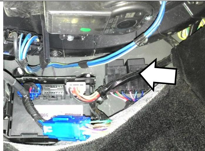
Route the remaining length of wires from the BD harness toward the driver's side or to the desired switch location.
