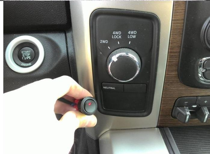
Using the stepper drill bit, create a hole to mount the switch. Use the small file to create a notch to locate the switch. The supplied decal may be used as a template.
