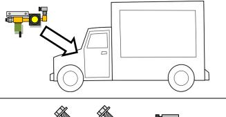
Route the air line/wire assembly from the air pump to the air regulator/solenoid assembly. Keep these lines away from the exhaust or sources of heat. Secure with zip ties to existing wiring harnesses or to the frame.
