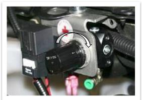
**NOTE** Over the next two weeks, the backpressure at idle may rise due to initial carbon build up on the inside of the brake housing and on the butterfly. The stop bolt may need to be adjusted again to compensate.
