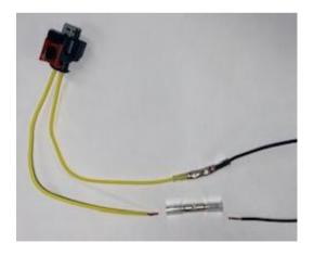
2. Connect new pigtail to injector
