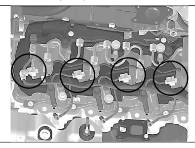
Disconnect old pigtail connector from injector and cut pigtail off of wiring harness.
