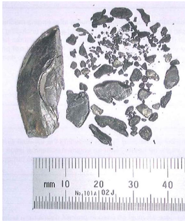
Figure 1 – Example of exhaust valve debris
